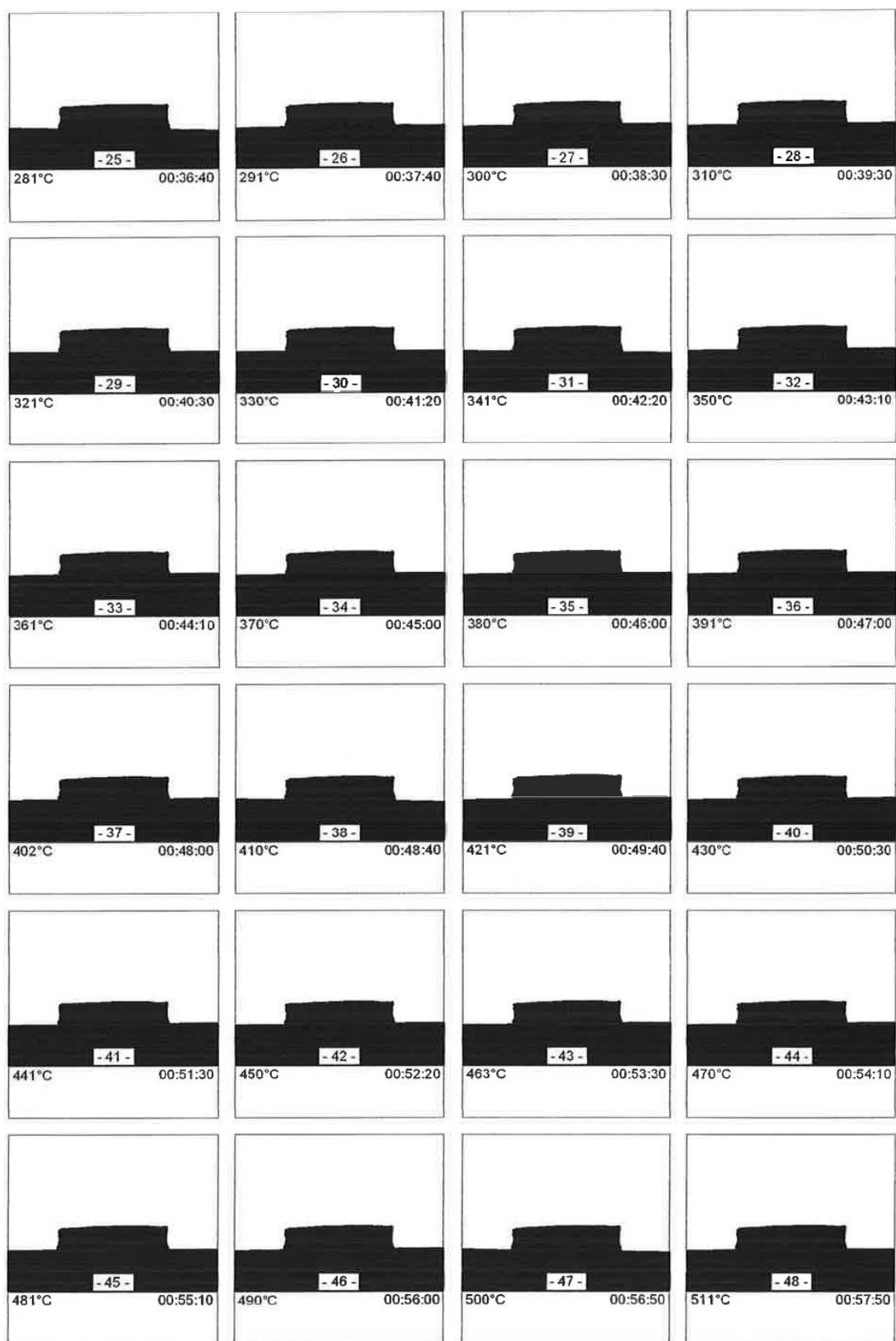
A. 46: Heating microscopy of PTC- \text{Al}_2\text{O}_3 prototype (280-510°C)
