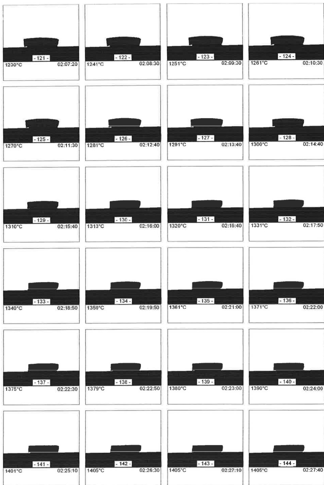
A. 44: Heating microscopy of PTC-BT-ZrO 2 prototype (1230-1400°C)
