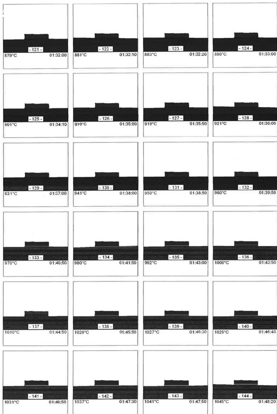
A. 30: Heating microscopy of thin PTC prototype (8800-1040°C)
