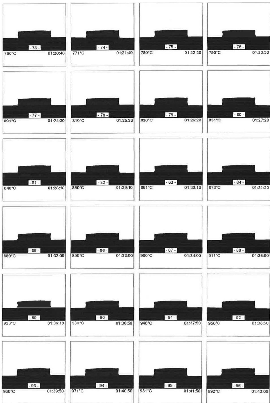
A. 48: Heating microscopy of PTC-Al 2 O 3 prototype (760-990°C)
