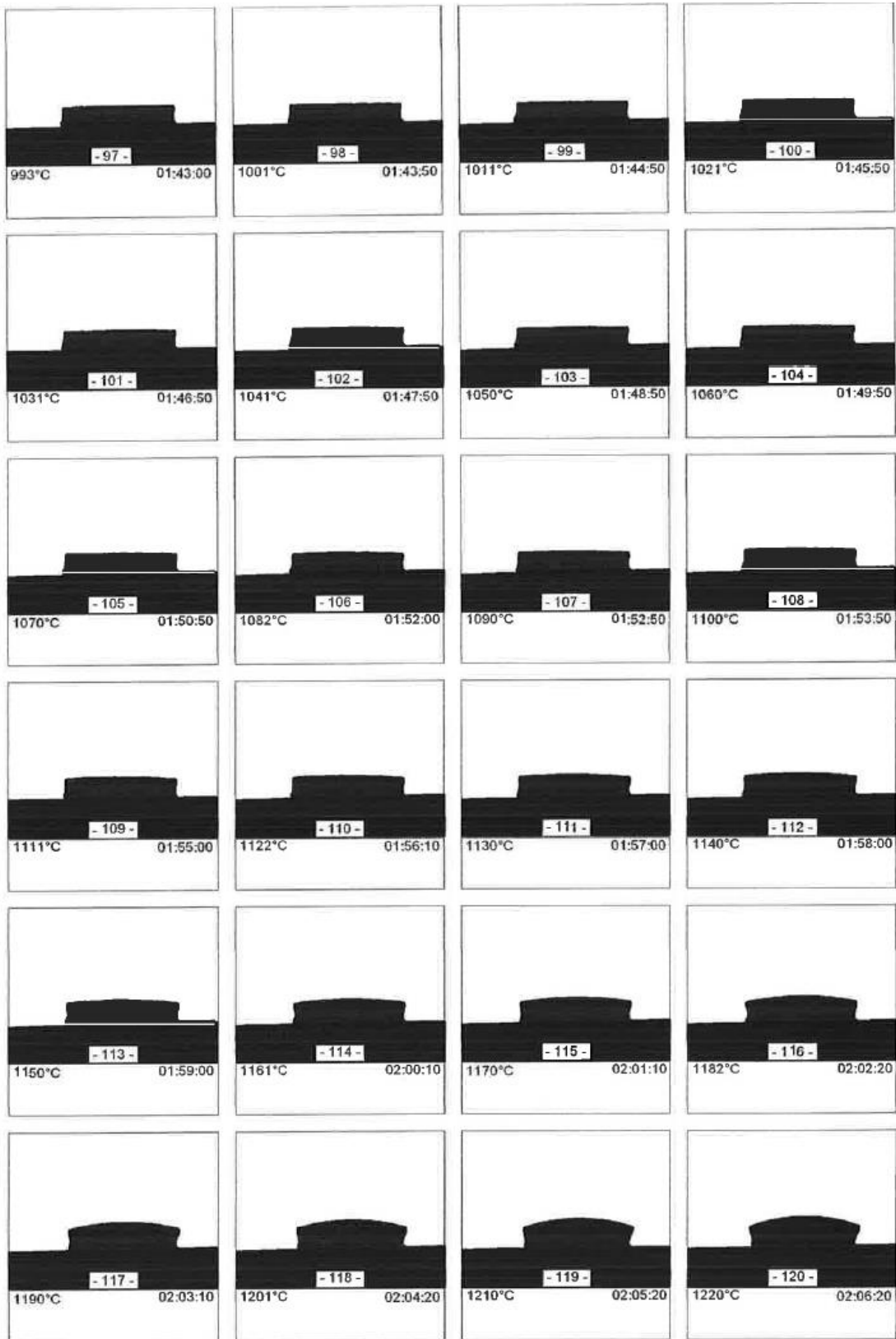
A. 37: Heating microscopy of PTC-ZrO 2 prototype (990-1220°C)
