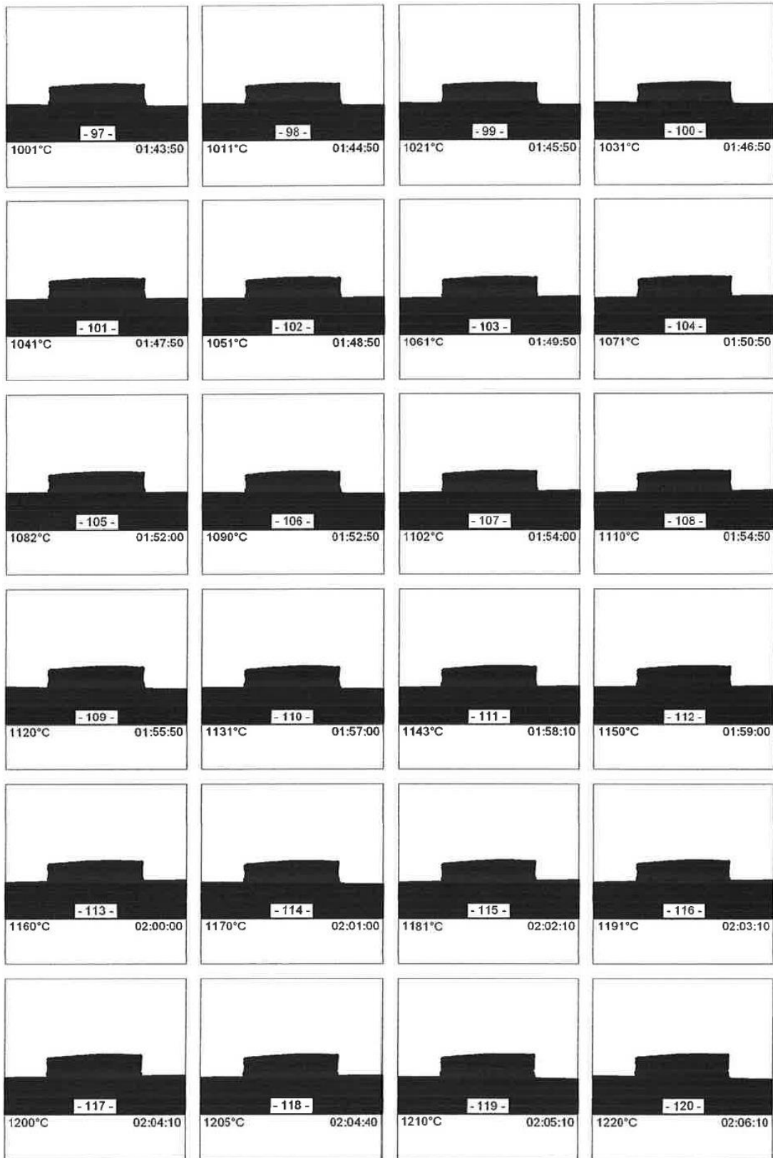
A. 49: Heating microscopy of PTC-Al 2 O 3 prototype (1000-1220°C)
