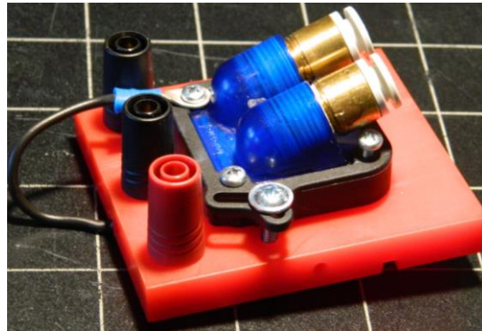
Figure 64: developed calorimetric measuring device
