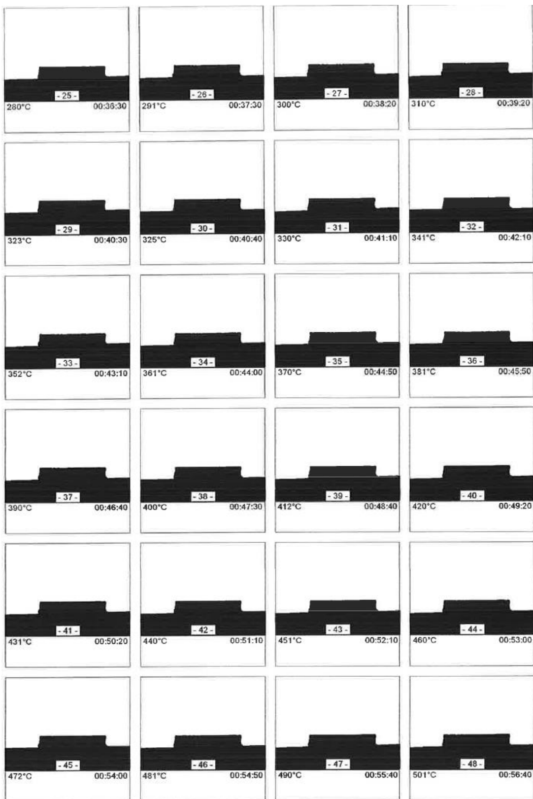
A. 34: Heating microscopy of PTC-ZrO 2 prototype (280-500°C)
