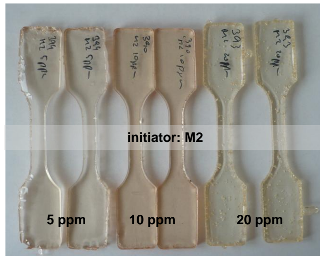
Figure 74: polyDCPD shoulder test bars (5, 10 and 20 ppm M2)
