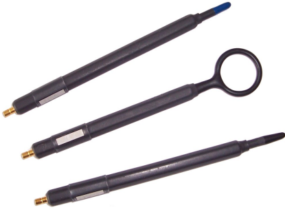
Figure 5.2: Near-field probes that have been used for the measurements.
