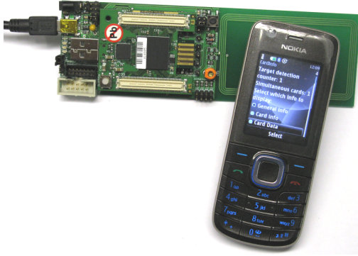
Figure 10.7: FPGA prototype communicating with an NFC-enabled mobile phone.
