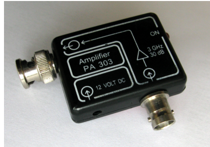
Figure 5.5: Picture of the 30 dB amplifier for the near-field measurements.
