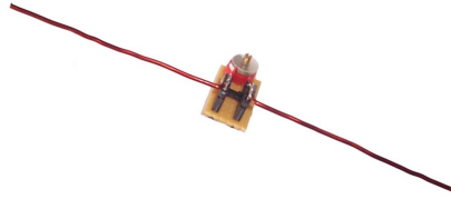
Figure 5.3: Self-made dipole antenna that has been used for the measurements.
