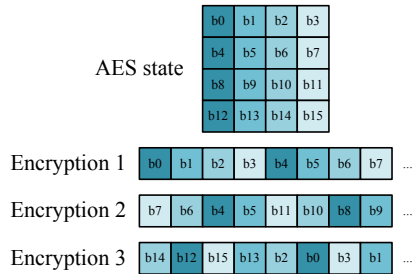
Figure 7.3: Principle of shuffling used in the randomized AES implementation.
