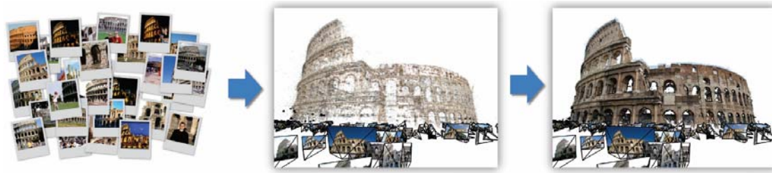
Figure 2.8: Workflow for geometry reconstruction from a community photo collection, as presented by S. Agarwal. Examples of user provided images with variable parameters (left), sparse 3D point cloud reconstruction acquired through SfM (middle) and the dense reconstruction using multi-view stereo algorithm (right) [Agarwal et al., 2010].
