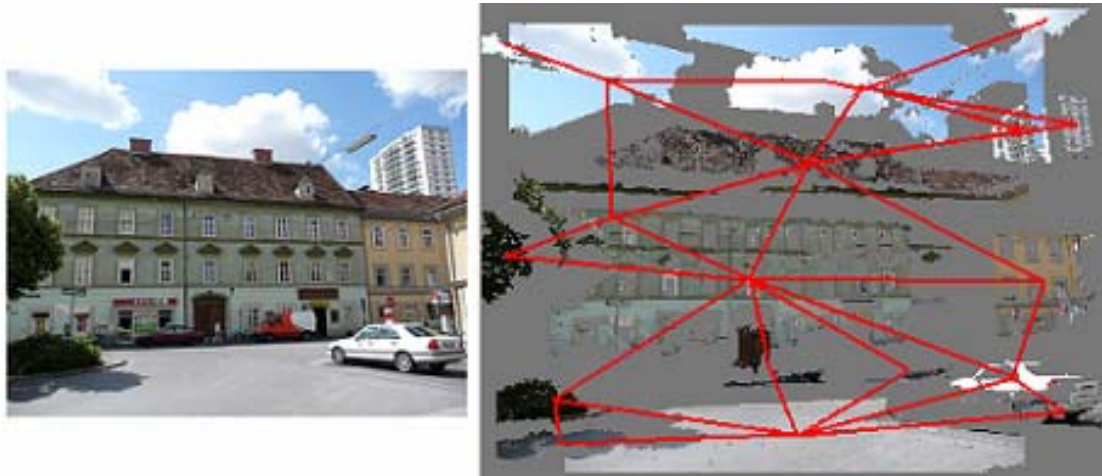
Figure 4.3: The example of the graph structure placed over the segmented image. Regions are represented as a graph node. An edge is placed between each two neighboring regions. This graph is the basic data structure for DRF and defines node areas as well as their neighborhood relationships. We can observe 19 nodes in the graph, each with 1-8 neighbors. In this example, only areas large than 15% of the image are displayed, as they represent significant objects in the image and are primary contributors for contextual relations.
