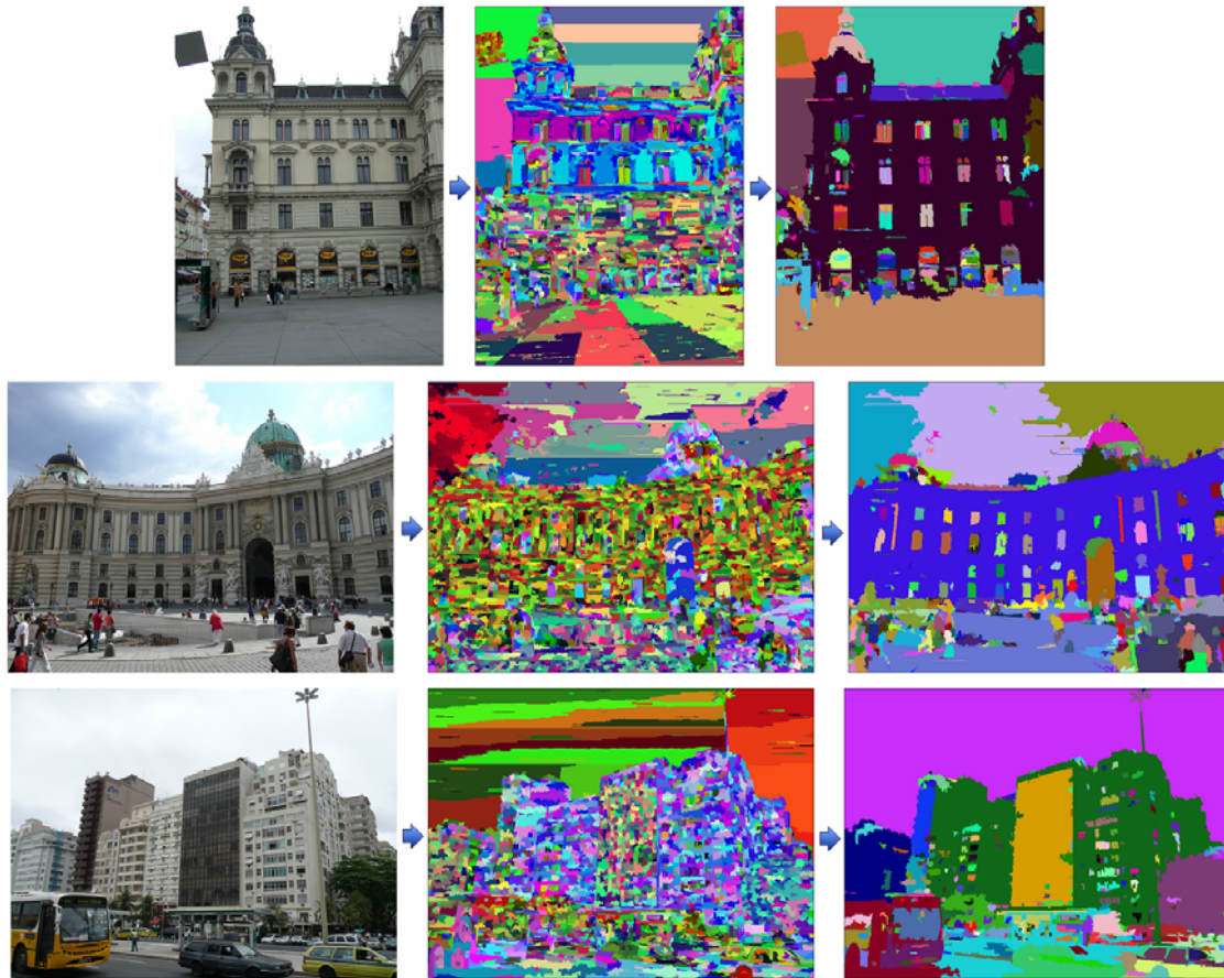
Figure 4.1: Segmentation examples represented in three steps described in this section. From the left: original image, over-segmentation from the watershed process that use texture as image primitive and the final segmentation after segment merging (segments are represented by a random color). Notice that in the final segmentation, the façades are represented only by one, or few large segments (even the covariance of the original façades varies greatly).
