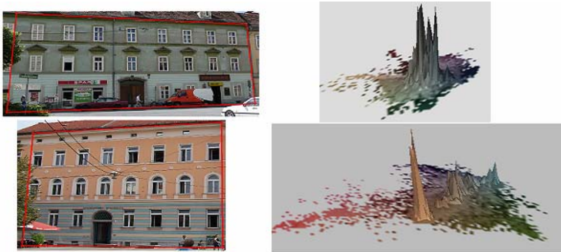
Figure 6.4: k-means clustering in CIE-Lab color space. Top row – façade with uniform color and it’s clustering visualization on the right side. The façade in the bottom row consist of areas with several different colors. This non-uniformity express by itself as several different clusters in a color space.
