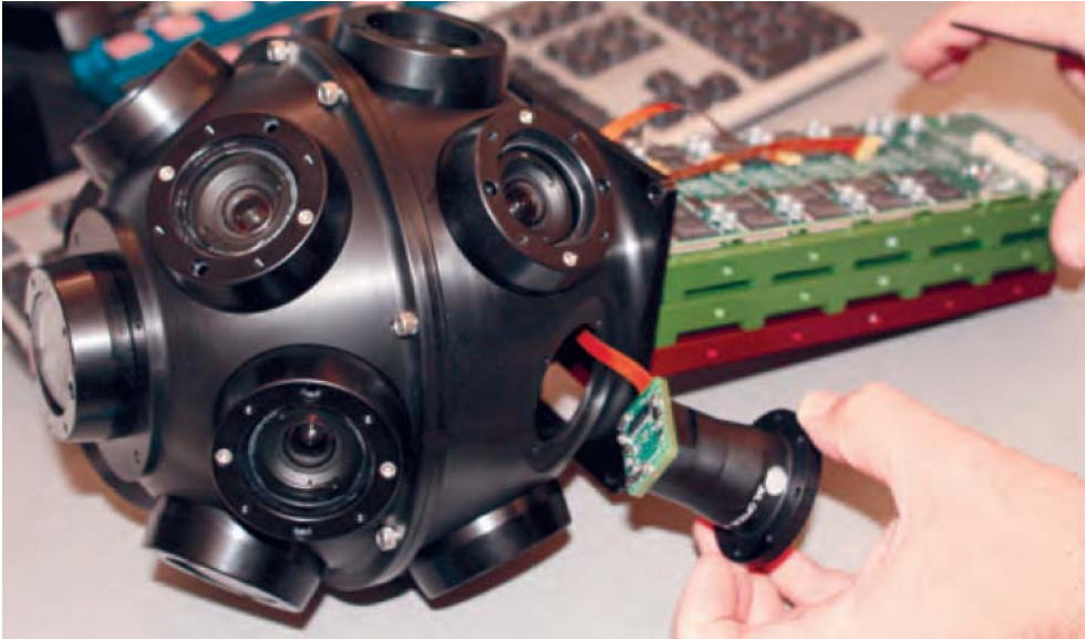
Figure 2.4: R7 camera system currently in development by Google. System is composed of 15 small, 5 Mpix CMOS sensors [Angelov et al., 2010].
