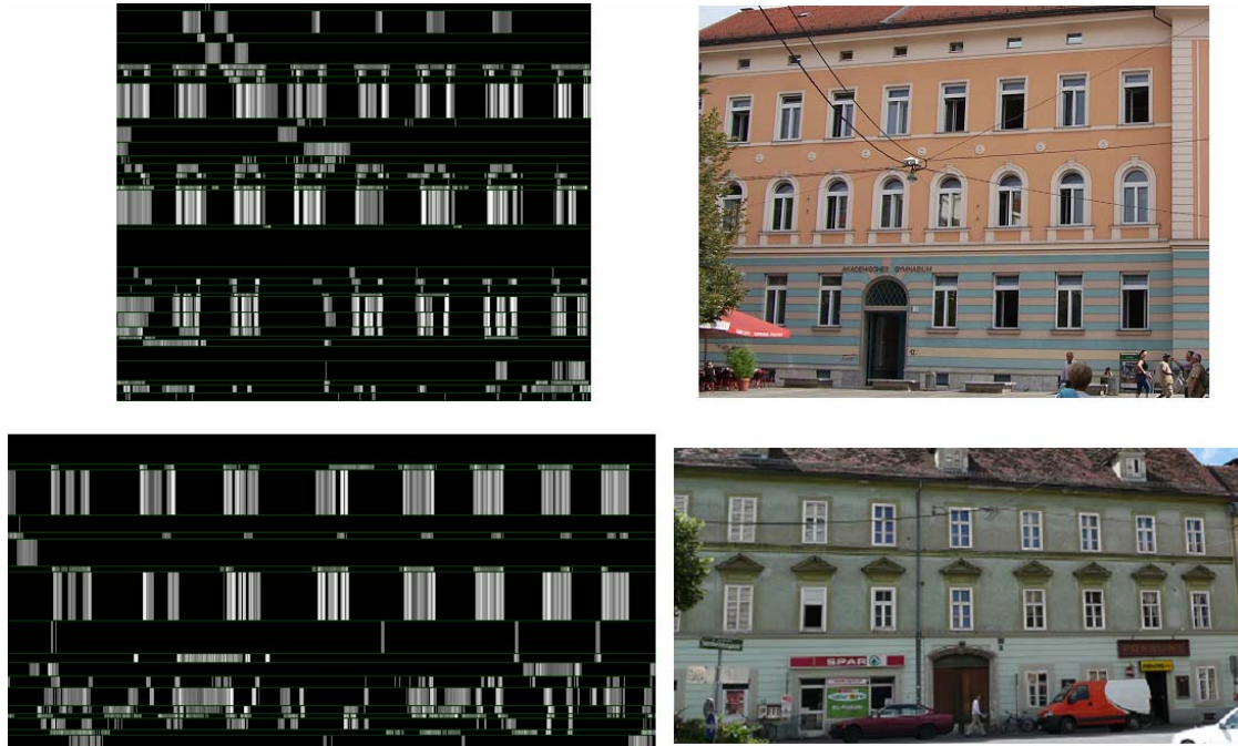
Figure 6.2: Gradient projection in our approach (on the left) and original façades (on the right). Horizontal projections are computed for each area between separator lines (green lines) independently. Value of the horizontal projection is visualized as an intensity of white lines.
