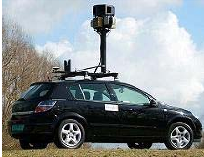
Figure 3.9: An example of a camera system mounted on a car. It is designed to cover wide viewing range.
