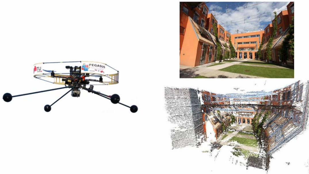
Figure 2.5: MAV system used for mapping of an urban environment (left) and the semi-dense point model obtained from refined sparse reconstruction from MAV’s data with original image from the scene (right) [Wendel et al., 2011].
