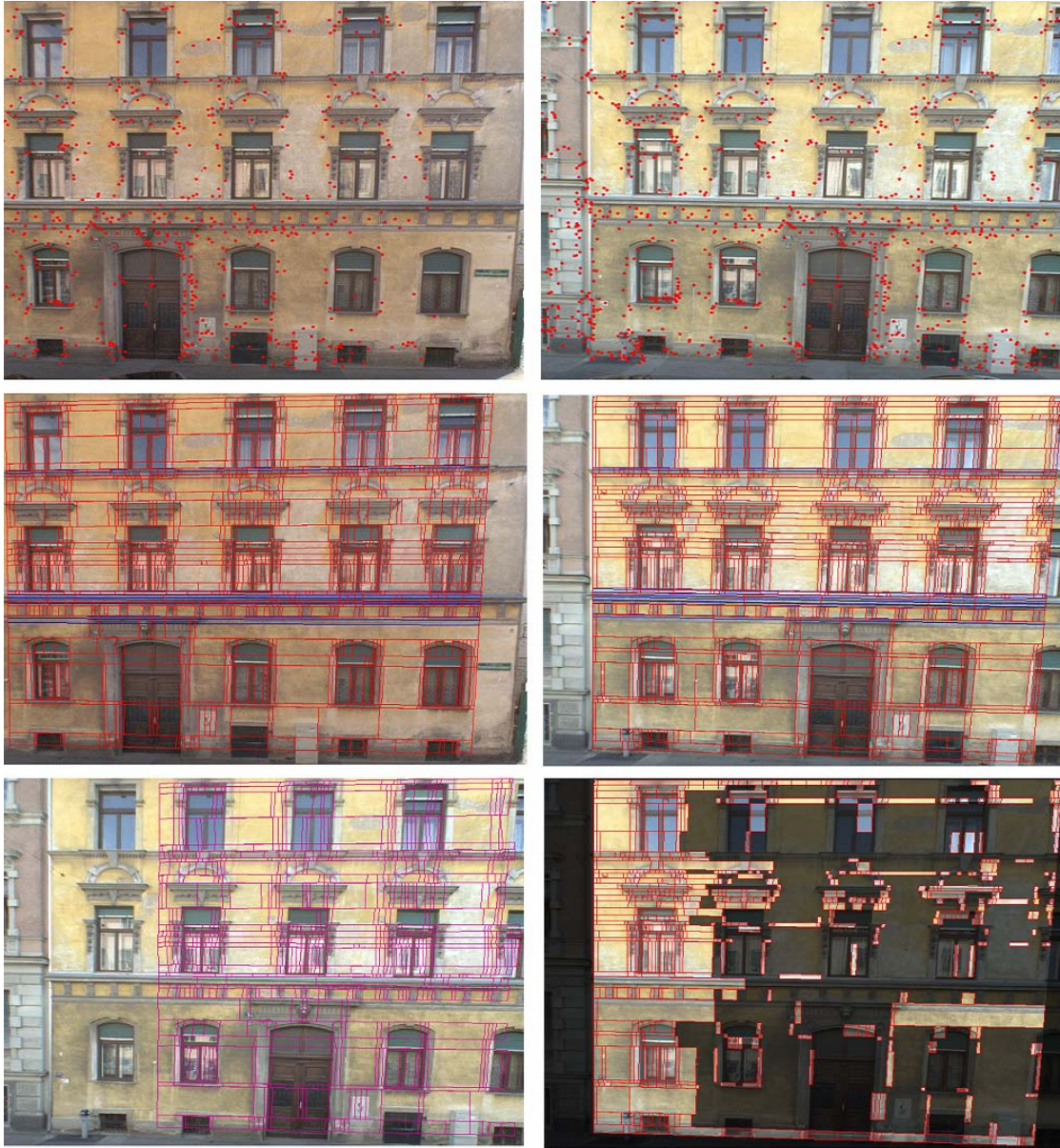
Figure 7.7: Two images of the same façade. Top row – matched corresponding points, middle row – blocks located in each façade, bottom row – blocks from first façade projected into second façade (on the left) and highlighted set of transferable sites (on the right). Notice the inaccuracies in projection of blocks between image (inclined edges of blocks) in bottom left image caused by imprecise matching of points. However these errors are not significant in computation of transferable sites.
