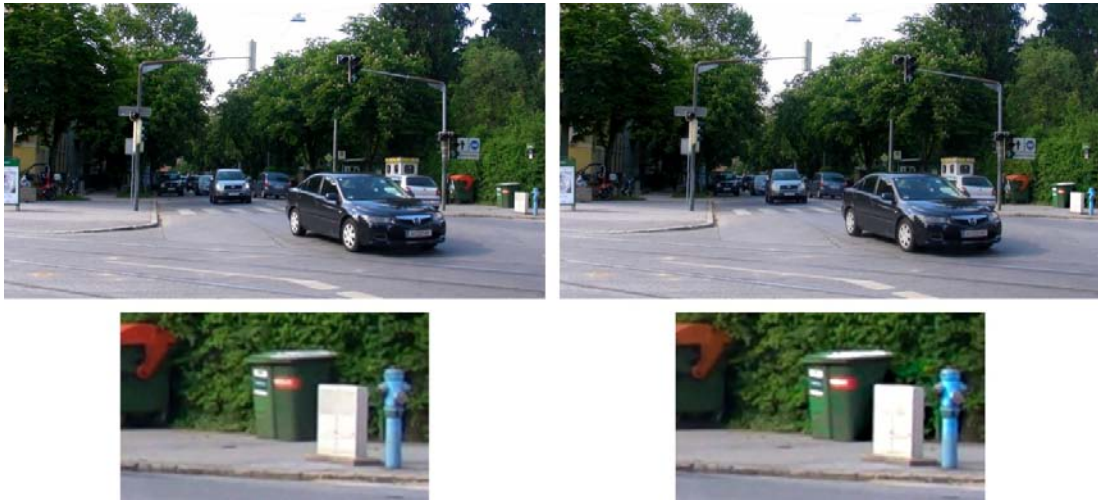
Figure 7. Attention direction example. (Top Left) Original capture image. (Top Right) Image after our modulation technique. The goal is to direct the attention to the far right trashcan and water pipe. (Bottom) Enlargements of the focus of interest.
