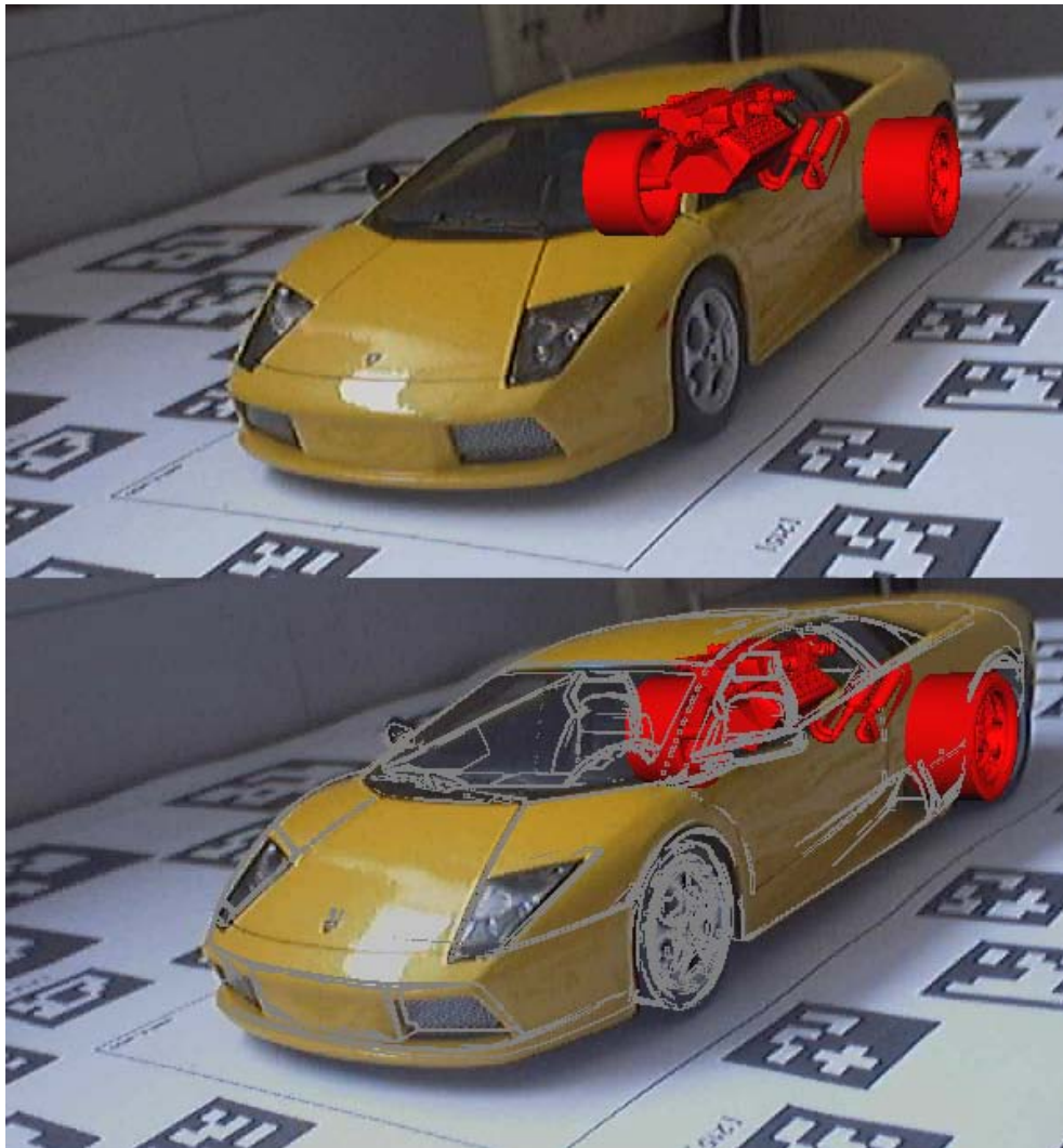
Figure 50. Using context from linked virtual models. (Top) This image depicts a crude augmentation of the car engine and back tires. (Bottom) This image shows that one can improve the perception of depth by adding hints at the locations of the important features of the context.
