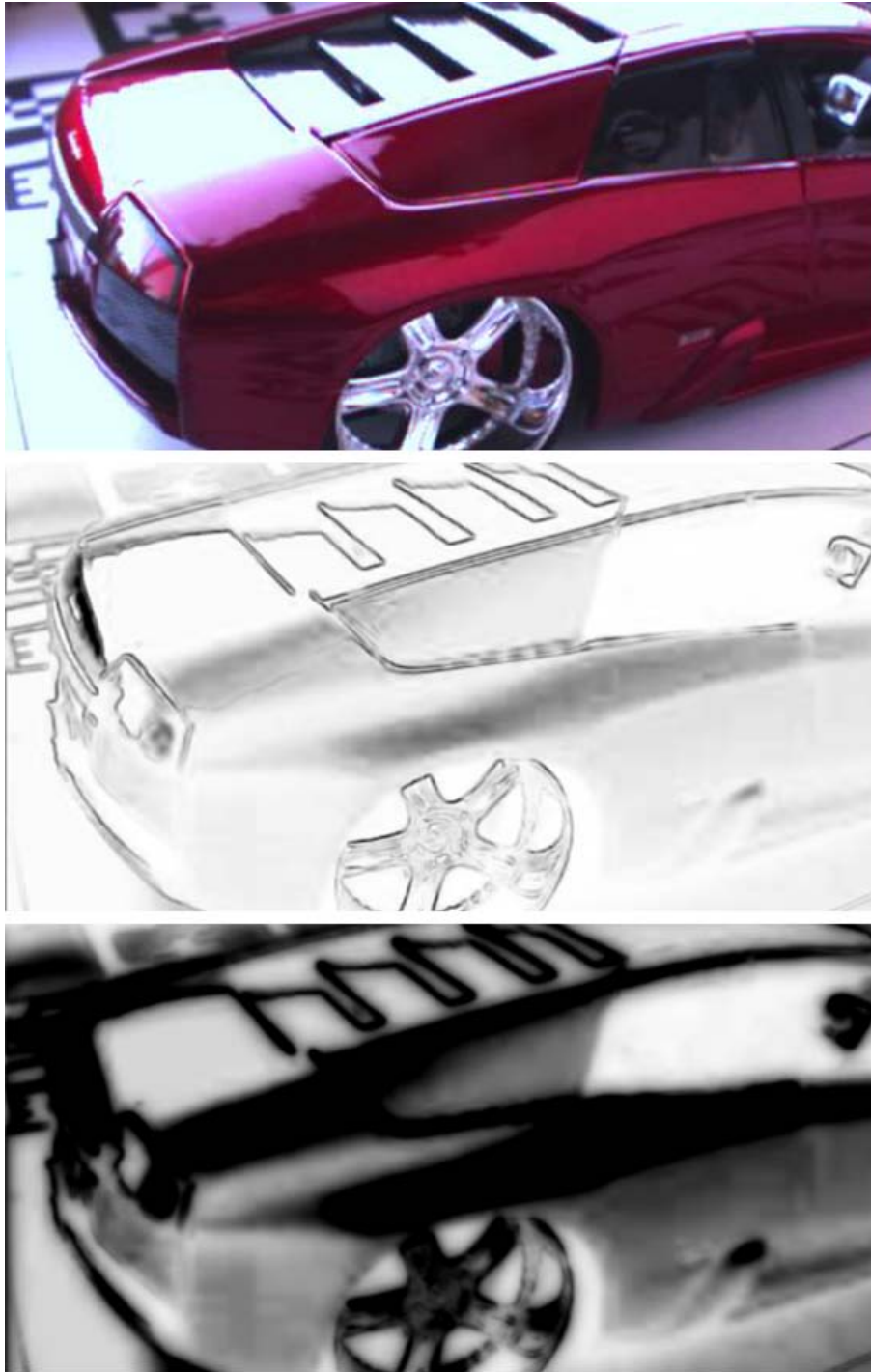
Figure 57. Haloed edges from variance. (Top) Original image. (Middle) Resulting edges (in black) from the image variance. (Bottom) Edges after haloing with the technique by Bruckner and Groeller (Bruckner and Groeller 2007).
