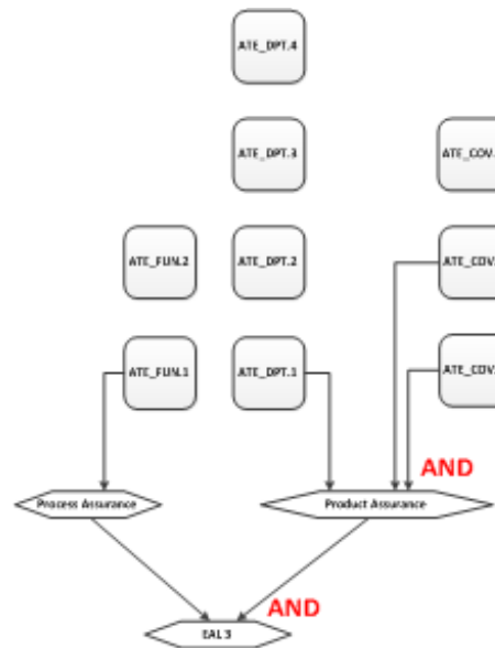
Figure 9. The current Common Criteria evaluation does not leave much room for flexibility. The hard goals are only fulfilled, if all (AND) inputs are true.
