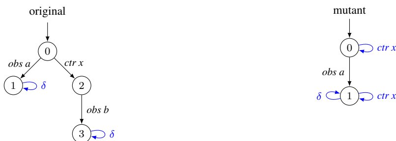
Figure 10.6: Two LTSs used for demonstration of differences between a pure ioco check and our combined refinement/ioco check, which are caused by the input-enabledness assumption of ioco.
