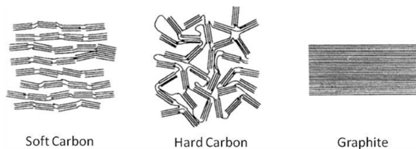
Figure 20: Schematic profile of the three different types of carbon (39)
