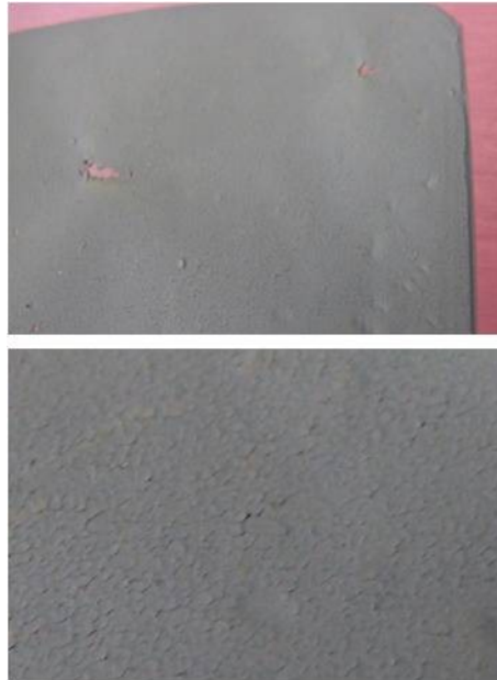
Figure 84: Picture of a silicon electrode-paste with a plasticizer coated on a copper foil
