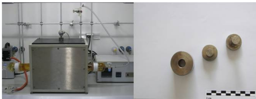
Figure 41: The glass tube furnace for preliminary alloying by solid state diffusion (left) and the special device to press pellets (right)
