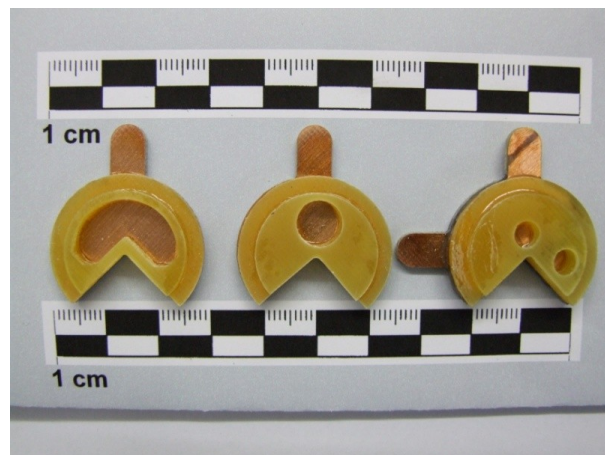
Figure 32: Various shapes of reference electrode adapters (counterpart circle segment not displayed)
