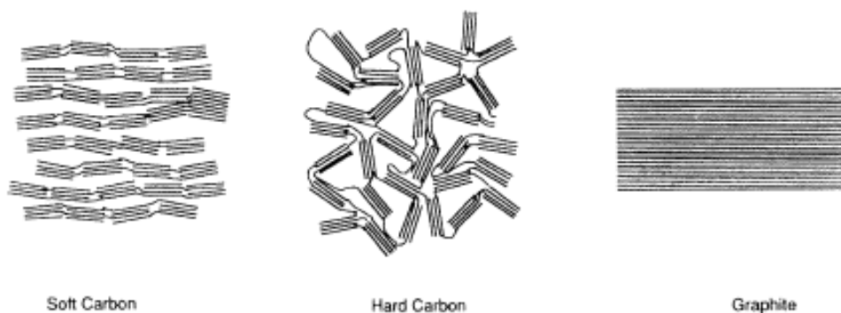
Figure 11: Structural differences of carbonaceous materials (29)
