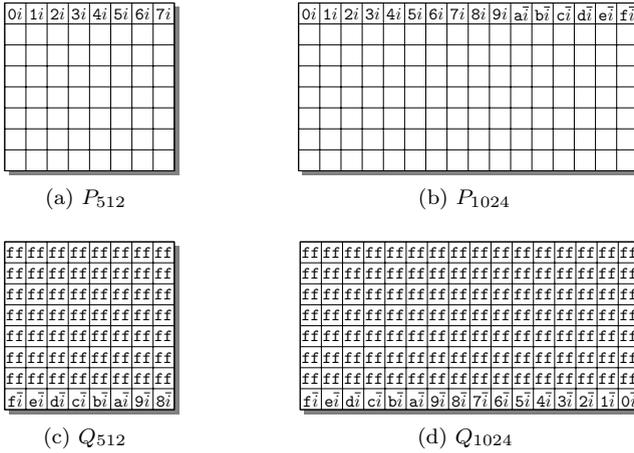
Figure 4.4: The XOR constants added by the AddRoundConstant transformation.
