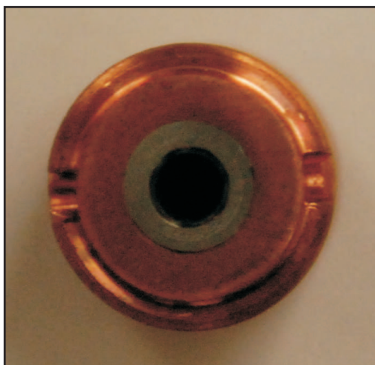
Figure 3.2: La sample - Lanthanum in the inner part of a copper cathode.
