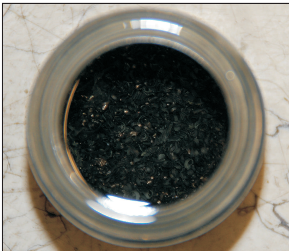
Figure 3.1: Pr sample - Praseodymium chippings stored in oil.
