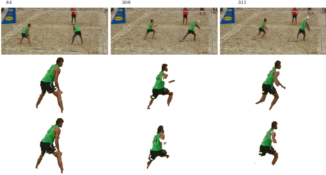
Figure 4.8: Comparison of anisotropic TV and standard TV regularization. The first row shows frames of the original video where the left player is tracked. In the second row the anisotropic regularization term shows a better segmentation of fast moving details than the standard weighted TV regularization in the third row.
