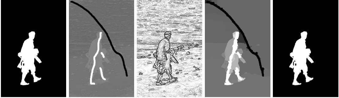
Figure 3.14: Example of image segmentation using the weighted ROF model. From left to right: The segmentation result using the continuous maximum flow algorithm (Algorithm 8). The unary potentials -c_u depicted in the interval [-0.05, 0.05] . The binary potentials c_b . The denoising result u . Finally, the segmentation obtained using the ROF model u > 0 .
