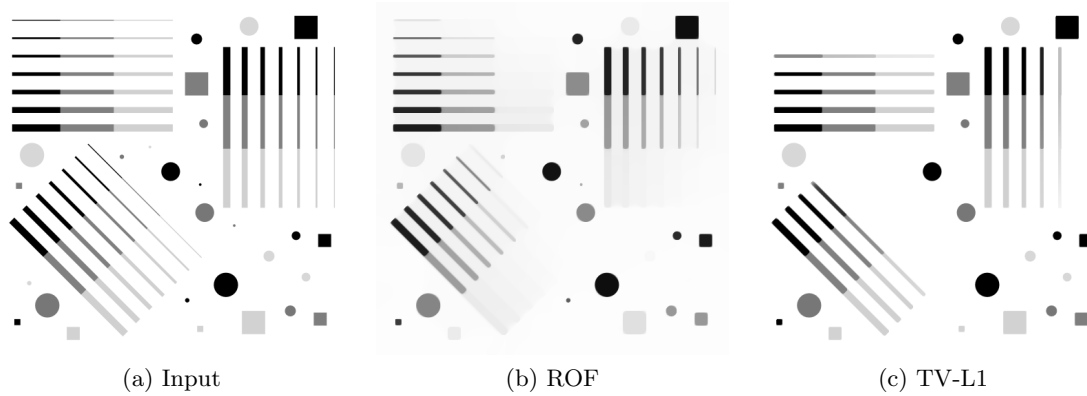
Figure 2.3: Demonstration of the contrast invariant denoising properties of the TV-L1 model (2.11), compared to the ROF model (2.9).
