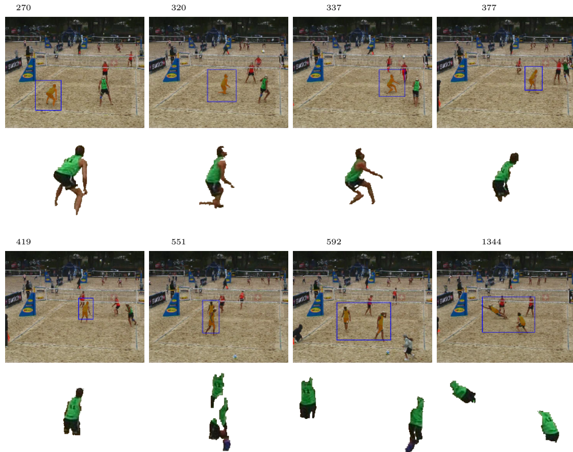
Figure 4.12: Tracking of volleyball sequence, where tracker fails due to highly similar object and colors in the background. The first row shows the input video and the bottom row shows the extracted player.
