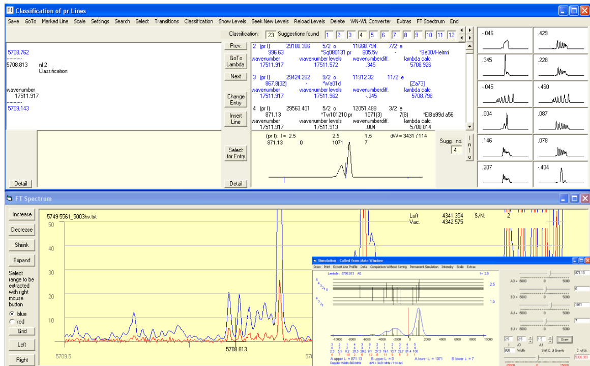
Figure 6.28: Predicted hf structure of the line 5708.813 Å.
