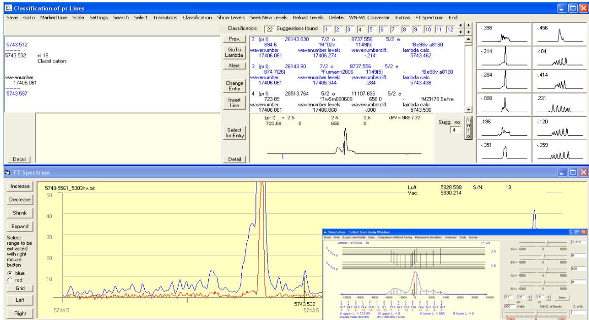
Figure 6.21: Predicted hf structure of the line 5743.53 Å.
