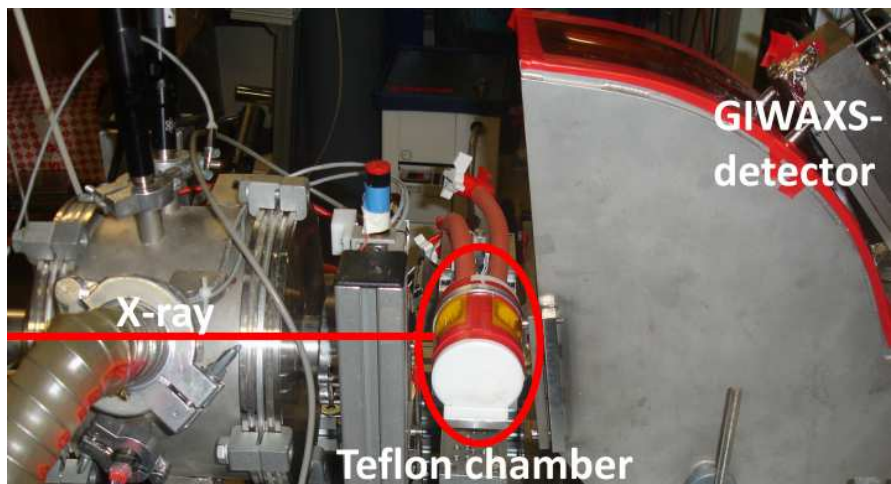
Figure 11: Special measurement chamber integrated into the GIWAXS measurement set up
