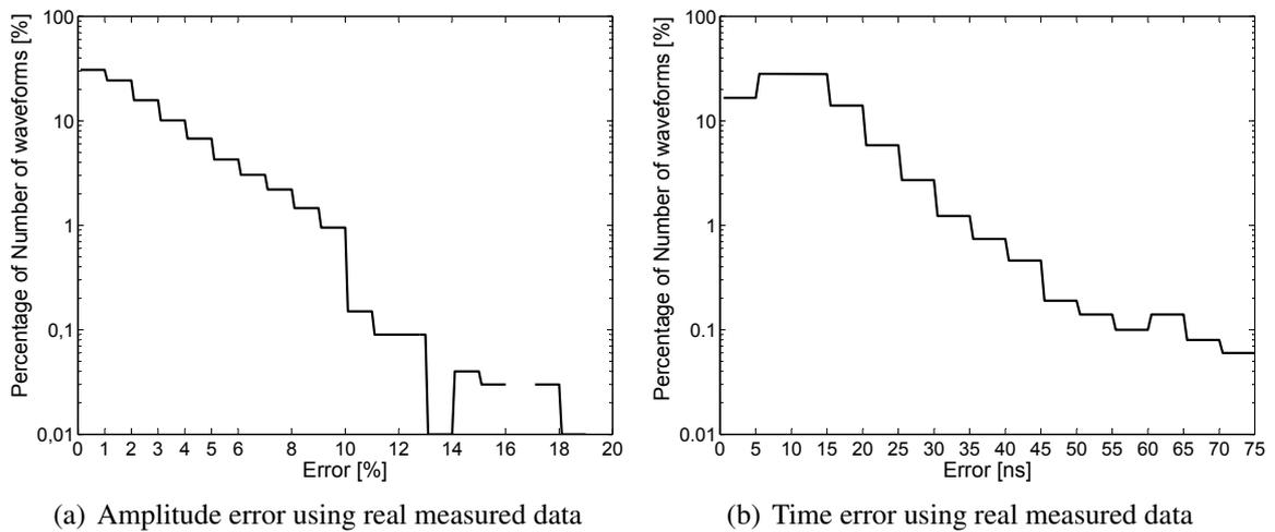
**Figure 4.29.:** Error in amplitude and time of the parameter extraction from 10 000 real measured waveforms from the test-data used in the previous compression methods. The amplitude error is given in percent of the differences normalized to the original amplitudes of the waveforms. The error in time is given in nanoseconds.
