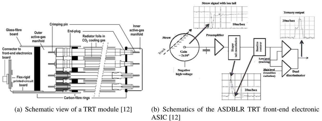
Figure 2.22.: Transition Radiation Tracker module and front-end of the ATLAS experiment
