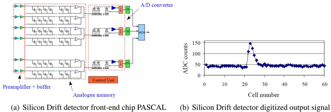
**Figure 2.9.:** ALICE silicon drift detector PASCAL ASIC and its output signal
