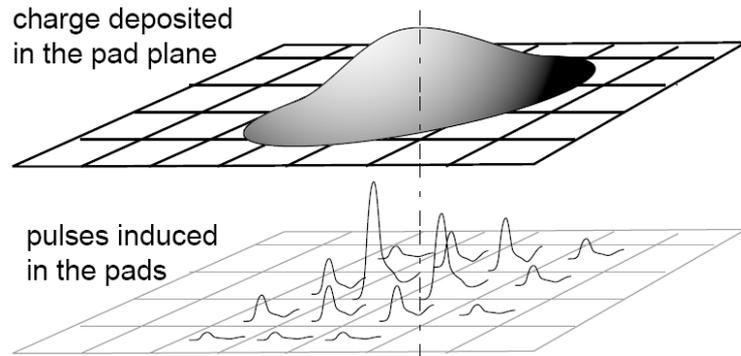
**Figure 4.5.:** Schematic of the charge cloud from the avalanche process in the MWPC of the ALICE TPC (top) together with the schematics of the induced signals in the detector pads underneath (bottom)
