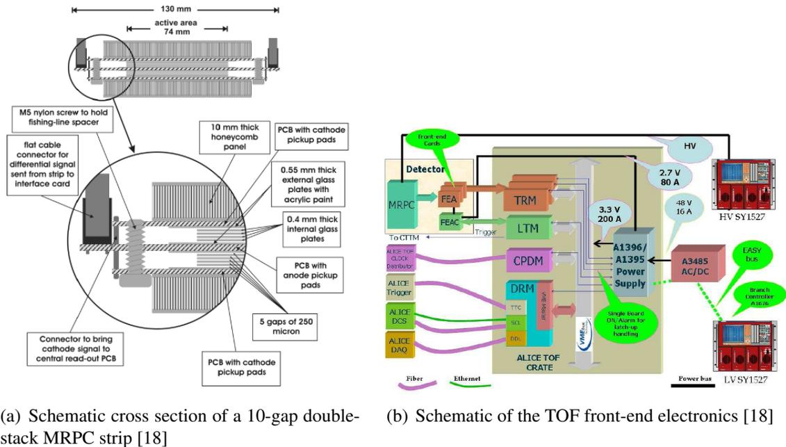
**Figure 2.24.:** ALICE Time-Of-Flight detector (TOF) Multi-gap Resistive Plate Chamber (MRPC) strip and the front-end electronics connected to the pick-up pads of the strips
