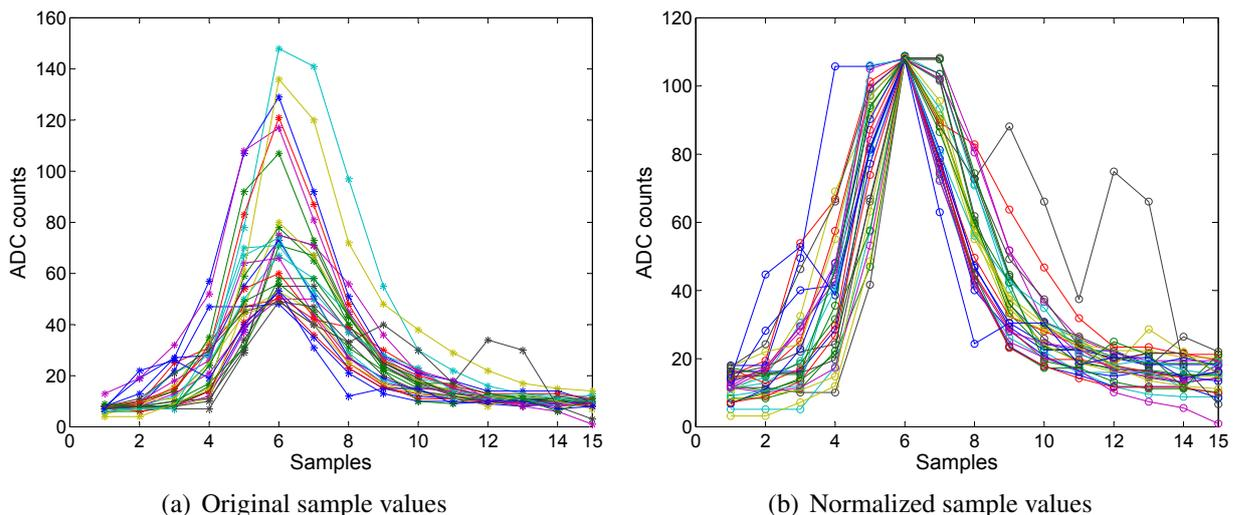
**Figure 4.7.:** Samples of first 30 input waveforms in the test-data matrix in original form and the normalized sample values
