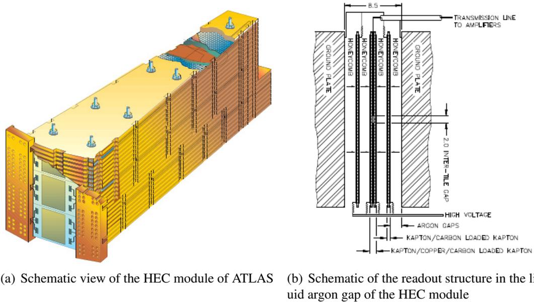
**Figure 2.14.:** ATLAS hadronic end-cap calorimeter (HEC) module [12]
