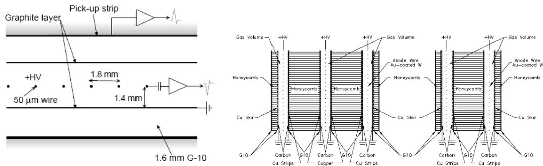
(a) Structure of a Tin Gap Chamber [12] (b) Cross-section of a TGC triplet and doublet module. The triplet has three wire layers but only two strip layers. The doublet has two wire and strip layers [12]
