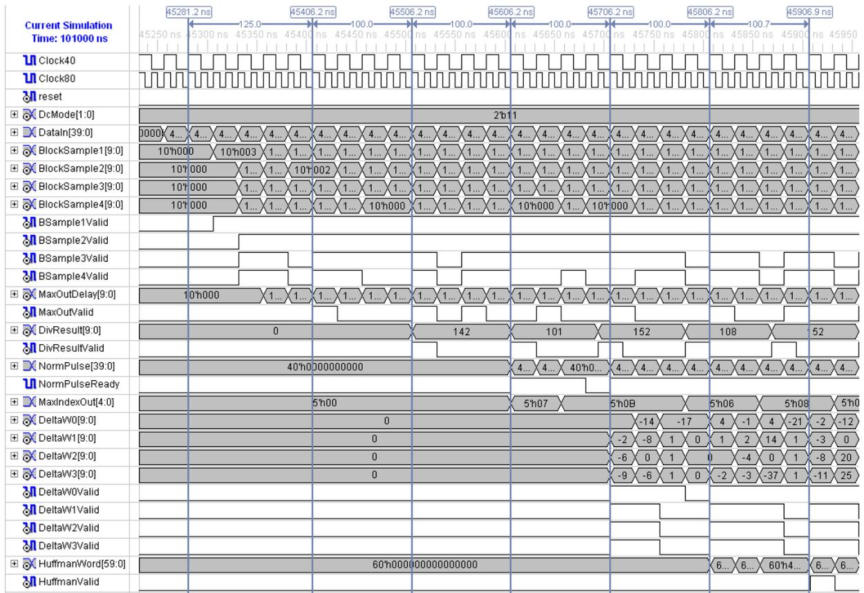
Figure 6.6.: Signal diagram used to investigate the latency of the DataCompressor
