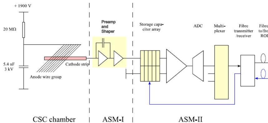
**Figure 2.29.:** Schematics of the CSC front-end electronics of the ATLAS experiment [12]
