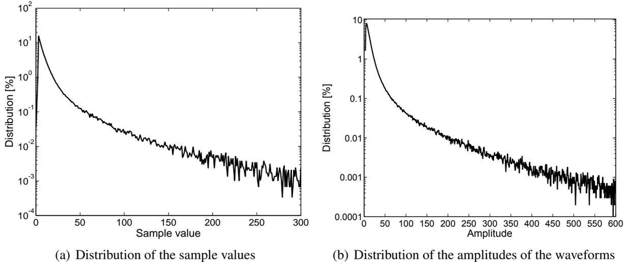
**Figure 4.4.:** Distribution of the sample values and amplitudes of real zero suppressed proton-proton collision waveforms measured from the TPC in ALICE in 2010
