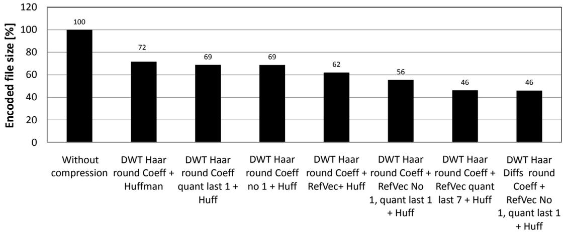
**Figure 4.22.:** Comparison of the compression ratios resulting from the various DWT methods with the Haar wavelet performed on the test-data from the ALICE TPC extended to 16 elements per input vector
