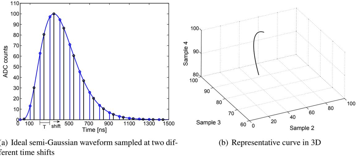
**Figure 4.26.:** An ideal semi-Gaussian waveform sampled at shifting sampling times of 5 ns in the range of  $[0, T]$  with a sampling period  $T$  of 100 ns. The resulting sets of samples are illustrated as points in a sample space. A 3-dimensional section of the sample space is shown using the samples 2, 3 and 4.
