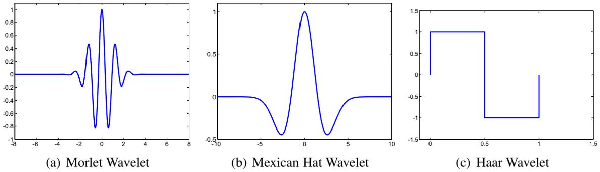
**Figure 3.12.:** Three examples of mother wavelet functions
