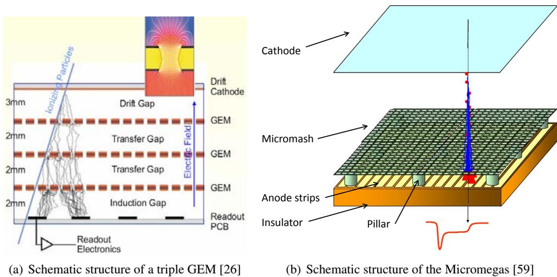
**Figure 7.4.:** Structural concept of GEM and Micromegas
