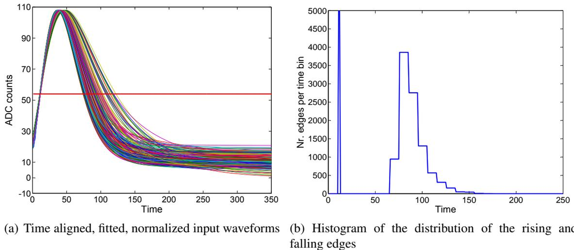
**Figure 4.10.:** The fitted input waveforms are oversampled and normalized and time aligned on their rising edge. The distribution of the points where the rising and falling edges cross the red line is shown in the histogram. The red line is positioned at half the maximum.
