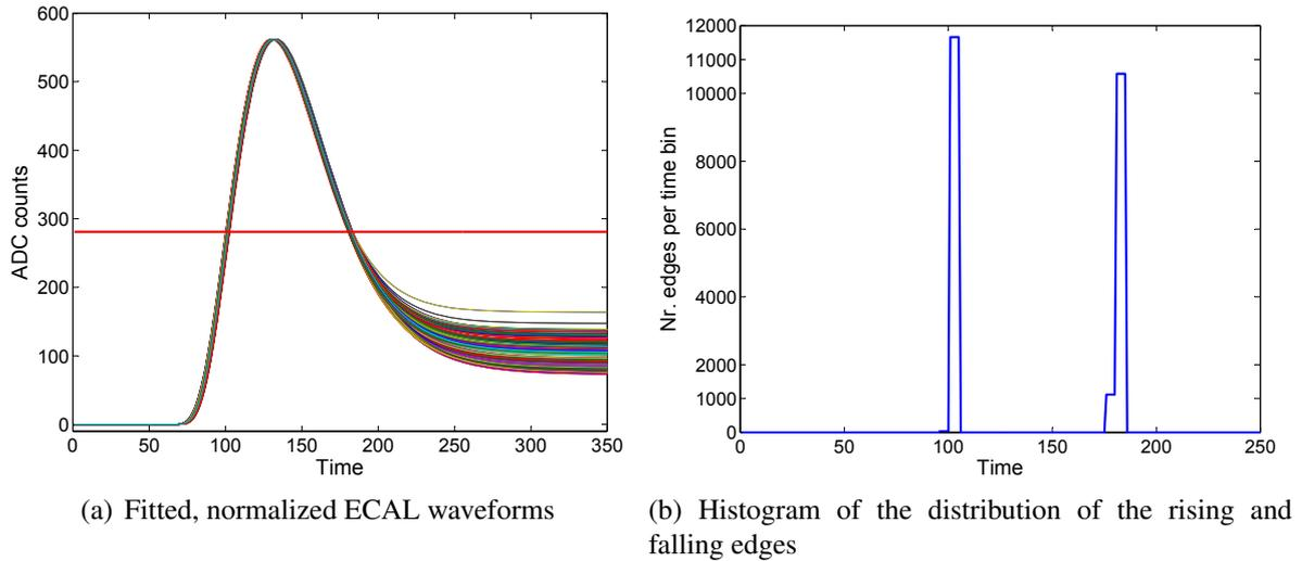
**Figure 4.12.:** Fitted input waveforms from ECAL data that are oversampled and normalized. The distribution of the points where the rising and falling edges cross the red line is shown in the histogram. The red line is positioned at half the maximum.
