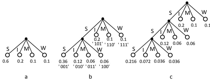
**Figure 3.2.:** Example of constructing a Tunstall tree
