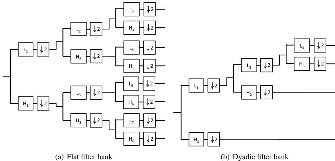
Figure 3.14.: Subband decomposition using 2 different filter bank concepts
