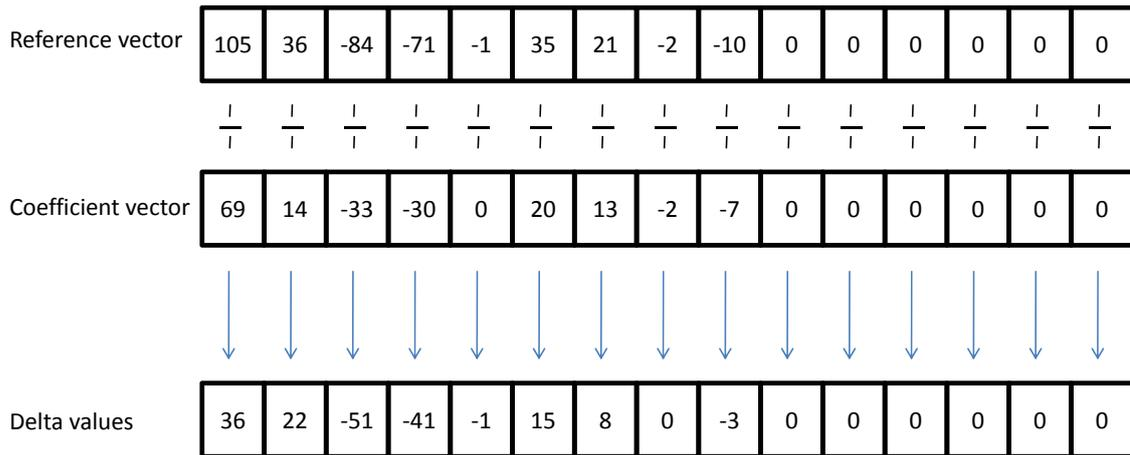
**Figure 4.16.:** Reference vector calculated from the mean of the coefficient vectors. One of the coefficient vectors is shown below the reference vector with the last six coefficients quantized to 0. On the bottom, the resulting delta values are given obtained from the subtraction of the coefficient vector from the reference vector
