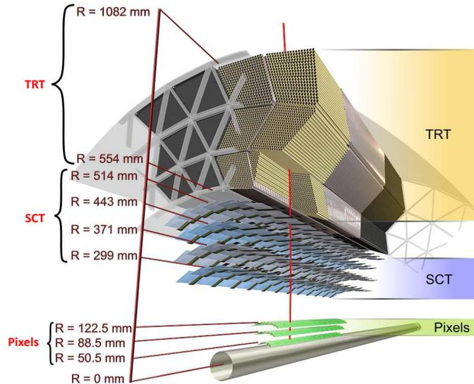
**Figure 2.3.:** The figure shows the inner detector layers of the ATLAS experiment and a horizontal charged particle track exiting the beryllium beam-pipe, in which the accelerated particles travel and collide. The several layers of pixel sensors, silicon microstrip sensors (SCT) and the transition radiation tracker (TRT), which surrounding the beam pipe at different radii provide the space points for the particle tracks passing through them [12]
