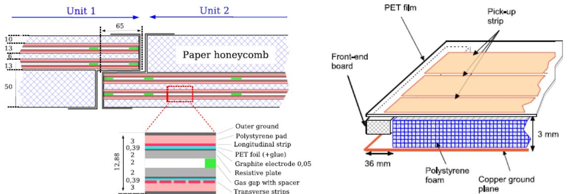
(a) Structure of the resistive plate chamber module composed of two units. Each unit has two RPC's. The cross-section of an RPC is shown at the bottom [12] (b) Layout of the RPC readout strip plane [12]
