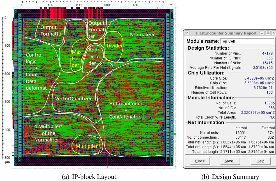
Figure 6.15.: DataCompressor IP block Layout and Design Summary
