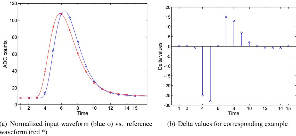
**Figure 4.8.:** Example of a normalized input waveform and a reference waveform constructed from the elements of a reference vector. The resulting delta values at the right have to be transmitted to prevent information loss.
