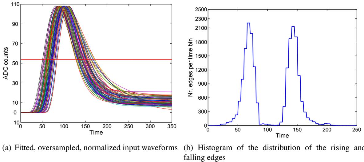
**Figure 4.9.:** The fitted input waveforms are oversampled and normalized. The distribution of the points where the rising and falling edges of the waveforms cross the red line is shown in the histogram. The red line is positioned at half maximum.
