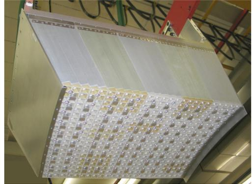
(b) Picture of the front view of the barrel ECAL of CMS
