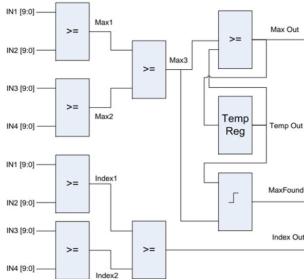
**Figure 5.7.:** Block diagram of the MaxFinder module, which uses combinational logic to search for the maximum sample value and the position of the maximum sample in the input waveforms
