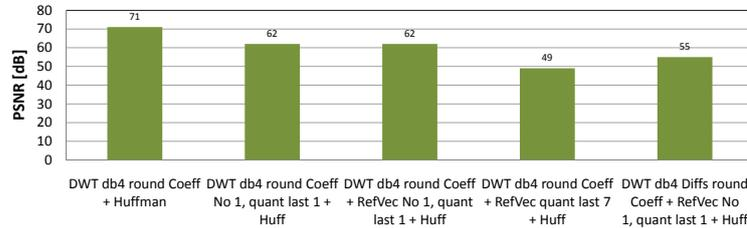
**Figure 4.25.:** Comparison of the peak signal to noise ratios ( $PSNR$ ) resulting from the introduced distortion of the various DWT methods with Daubechies 4 wavelet performed on the test-data from the TPC
