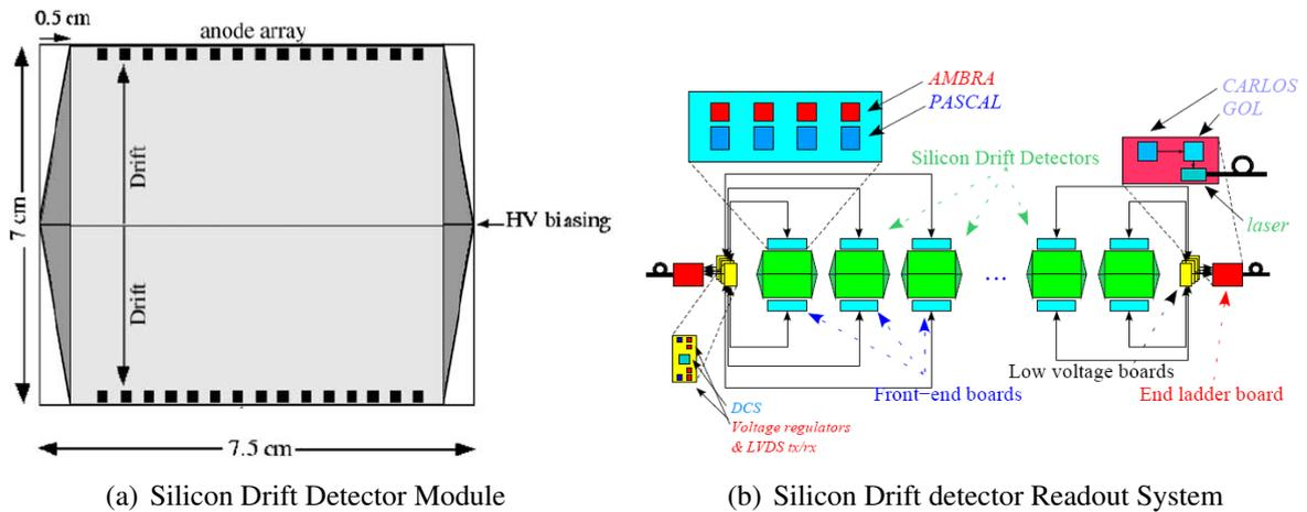
**Figure 2.8.:** ALICE silicon drift detector module and readout system containing PASCAL, ALBRA, CARLOS
