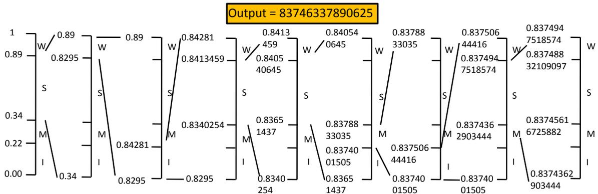
Figure 3.5.: Arithmetic Decoding: narrowing of the interval
