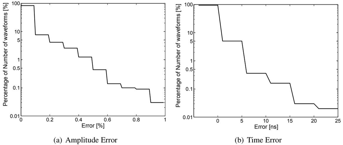
**Figure 6.7.:** Histogram of the error in amplitude (left) and time (right) between the reconstructed waveforms and the original waveforms. The error in amplitude is given in % of the original amplitude and the error in time is given in nanoseconds. The number of waveforms corresponding to the error is given in % of the total analyzed waveforms
