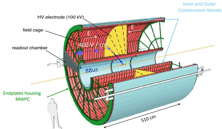
**Figure 1.2.:** ALICE Time Projection Chamber [1]
