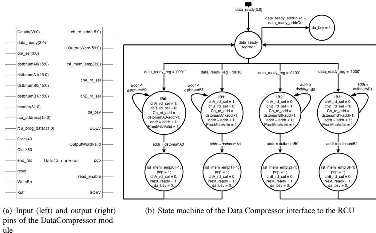
Figure 5.6.: DataCompressor module and input interface state machine
