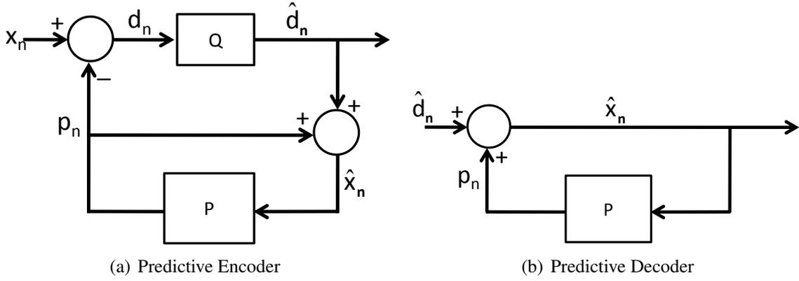
**Figure 3.15.:** Blockdiagram of the predictive coding method
