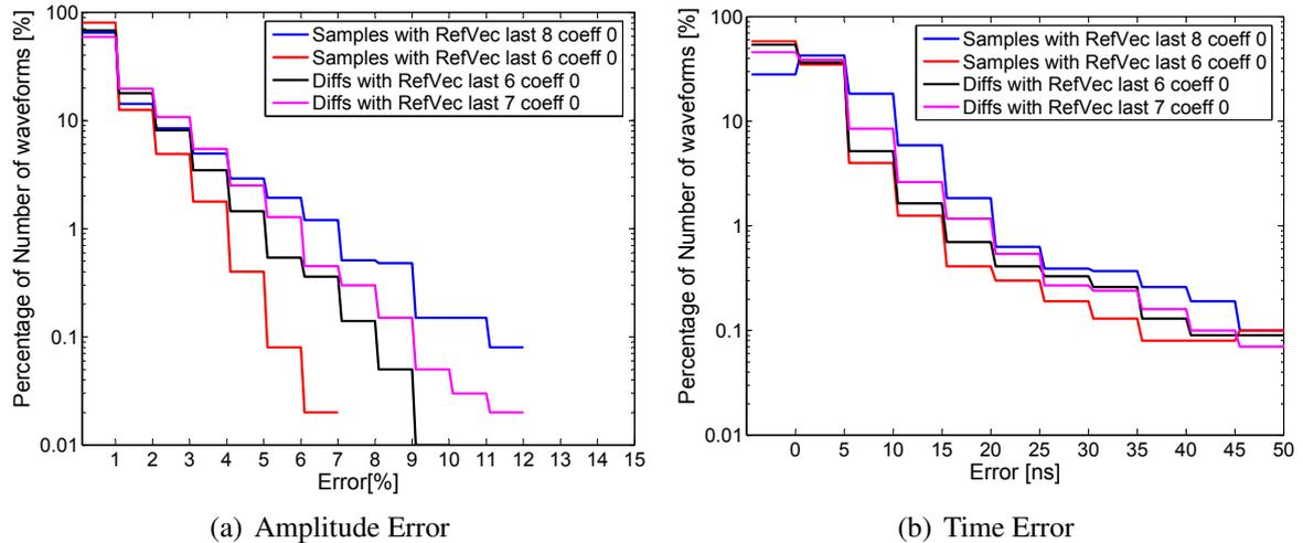
**Figure 4.17.:** Histogram of the error in amplitude (left) and time (right) between the original waveforms and the reconstructed waveforms from the DCT. The deviation in amplitude is given in % of the original amplitude and the error in time is given in nanoseconds. The number of waveforms corresponding to the error is given in % of the total analyzed waveforms
