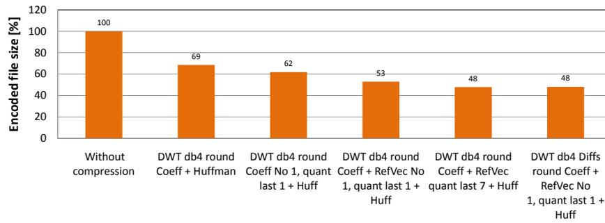
**Figure 4.24.:** Comparison of the compression ratios resulting from the various DWT methods with the Daubechies 4 wavelet performed on the test-data from the TPC extended to 16 elements per input vector
