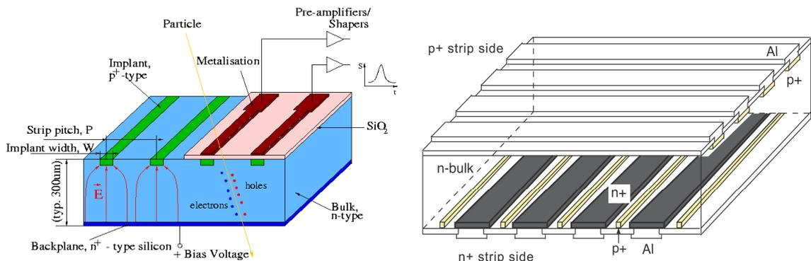
(a) Principle of a silicon strip detector [15]
