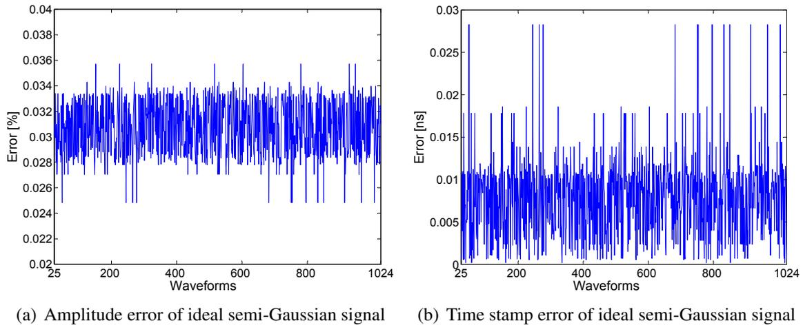
**Figure 4.28.:** Error in amplitude and time of the parameter extraction from 1000 ideal semi-Gaussian signals with different amplitudes and sampling times. The amplitude error is given in percent of the differences normalized to the original amplitudes of the waveforms. The error in time is given in nanoseconds.
