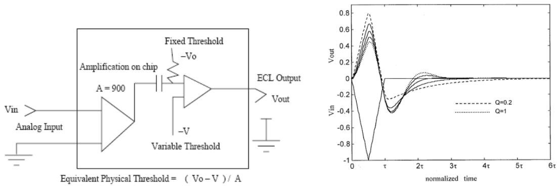
(a) Schematics of the front-end electronics [29] (b) Shaped output signal of the Amplifier/Shaper stage [30]
