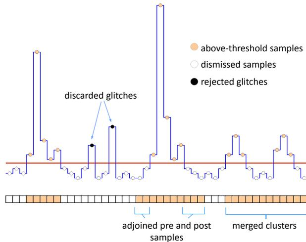
**Figure 5.2.:** Zero Suppression in the ALTRO chip [3]
