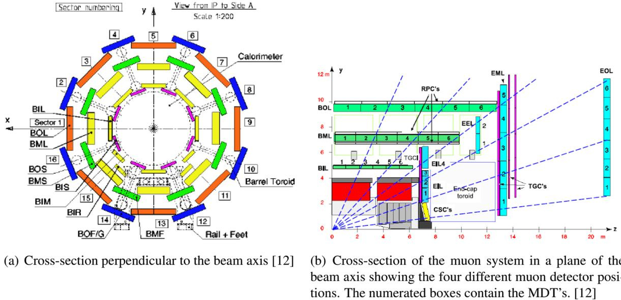
**Figure 2.25.:** Layout of the ATLAS muon system composed by Monitored Drift Tubes (MDT), Cathode-Strip Chambers (CSC), Resistive Plate Chambers (RPC) and Thin Gap Chambers (TGC)
