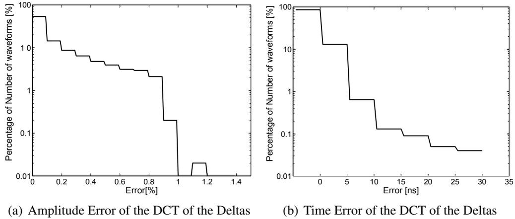
**Figure 4.18.:** Histogram of the error in amplitude (left) and time (right) between the original waveforms and the reconstructed waveforms from the DCT of the deltas from the lossless vector quantization method. The error in amplitude is given in % of the original amplitude and the error in time is given in nanoseconds. The number of waveforms corresponding to the error is given in % of the total analyzed waveforms.
