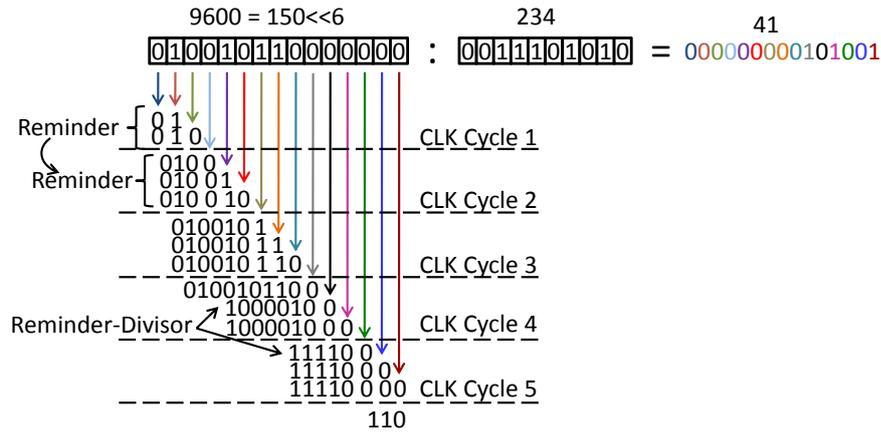
Figure 5.8.: Pipelined integer divider with five pipeline stages
