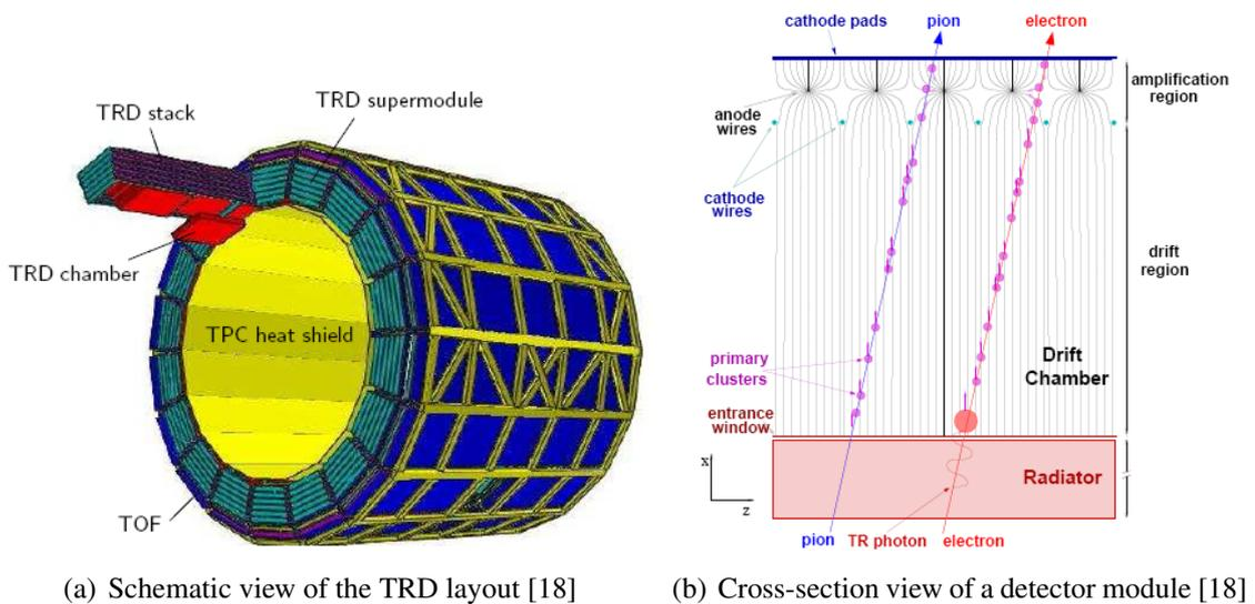
**Figure 2.20.:** Transition Radiation Detector of the ALICE experiment
