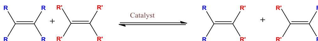
Scheme 1.1: Olefin metathesis reaction of two different olefins
