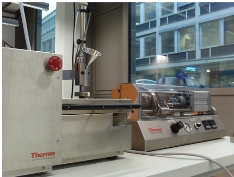
Figure 6-1: Haake MiniLab Micro Compounder (left) and DSM Research Injection Molding Machine (right).
