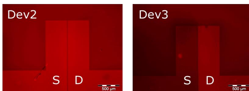
Figure 6.11: Fluorescence image of the source/drain electrodes of a P3HT EGOFET after contacting with 0.01 M NaCl in DI H 2 O (Dev2) and recording transfer and output characteristic (Dev3) gated via Pt and Ag/AgCl.
