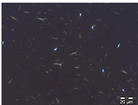
Figure 6.14: Dark field microscope image of a P3HT film on glass (without HMDS coating) after exposure to water.
