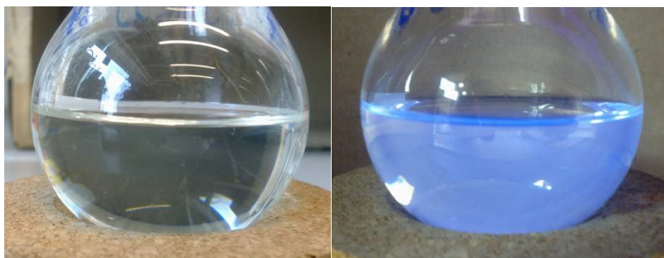
Figure 21. Cross-coupled caffeine 117 in a dichloromethane/methanol mixture at visible light (left) and by excitation at 366 nm (right).
