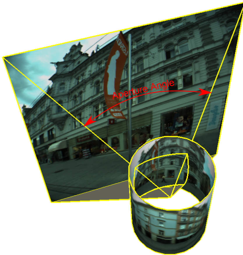
Figure 7.2: Panoramic Mapping of the environment onto a cylindrical surface. We use the term angular aperture to describe the FOV of a camera.
