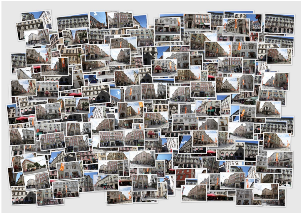
Figure 2.5: A larger high resolution image collection. To reconstruct the scene all image pairs have to be matched. Matching these pairs scales quadratically with the number of images, so efficient approximations become necessary.
