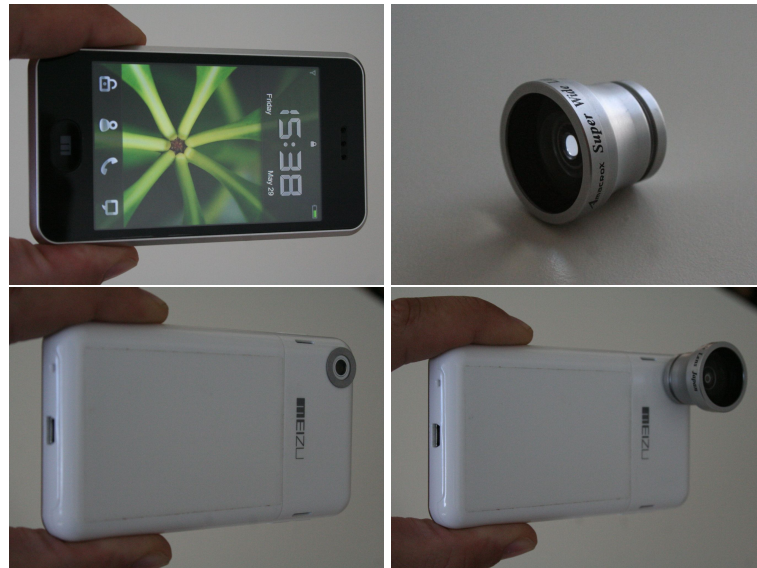
Figure 6.7: Meizu M8 mobile phone front view, back view with magnetic mounting ring, wide angle camera lens from AmacroX, mounted camera lens (from upper left to lower right).
