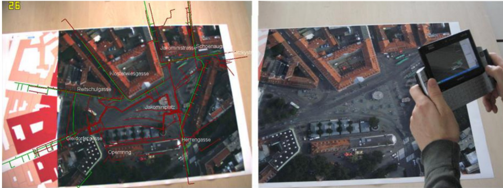
Figure 1.1: Augmented Reality User Interface for a Map. The user is equipped with a mobile device that renders 3D structures and information directly on top of the orthographic photo. The left image shows the screen of the mobile device, the user interaction is visible in the right image.
