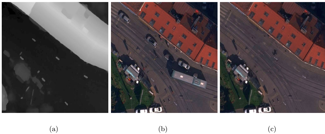
Figure 1.7: This Figure shows ortho images composited from multiple input images using the DSM (a) as a reference surfaces. Even though the DSM is not a true 3D data structure, its geometry can be used to generate a high quality true ortho image as the error caused by roof overhangs and similar truly three dimensional structures is minimal. Ortho image (b) is produced by a labeling and stitching approach, whereas (c) was obtained by estimating the continuous color surface.
