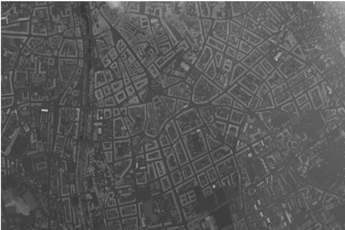
Figure 1.6: A digital surface model derived by fusing all available range images into one height field using the method proposed in this thesis.
