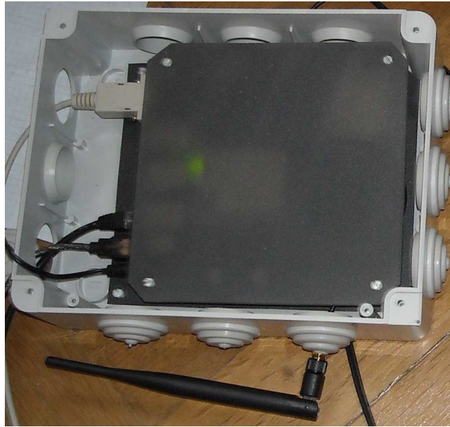
Figure 5.2: Alix board with open front plane.
