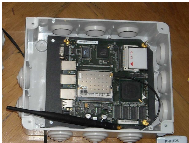
Figure 5.1: Alix board with open front plane.
