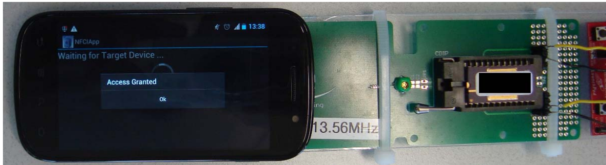
Fig. 12. This picture shows the NIZE prototype assembly. The NFC reader (Samsung's Nexus S) is put upon the target device's antenna circuit. It powers the target device's NFC interface chip and communicates with the access control terminal (RoTD).
