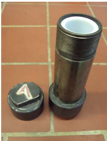
Figure 34: Teflon-coated steel autoclave for diatomite alteration experiments
