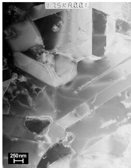
Figure 4.36: Transmission electron microscopy image of HPT-Cu B with 3 revolutions in radial direction annealed at 420 K. The magnification is 17 500.
