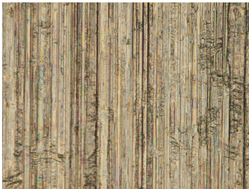
Figure 2.60: Finished hexaphenylcyclotrisilazane coat on a steel plate; resolution 1:50 000
