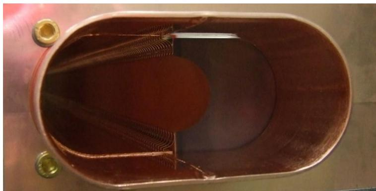
**Figure 5.19:** TCDQ aperture (courtesy W.Weterings).
