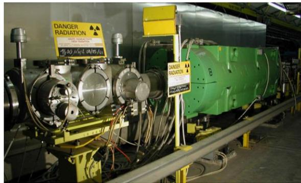
Figure 4.7: Internal SPS TIDV dump element (green) with beam instrumentation tank in front.
