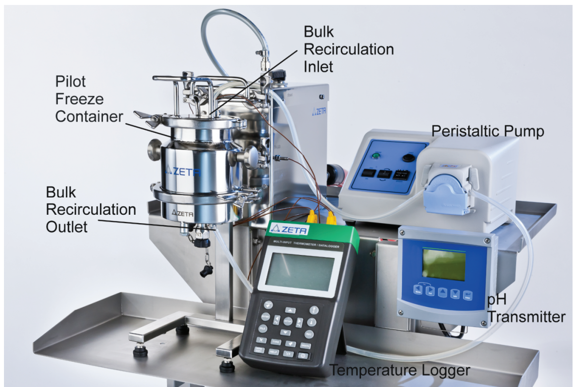
Figure 1: Pilot freeze container system overview; external freeze controller is not shown.
