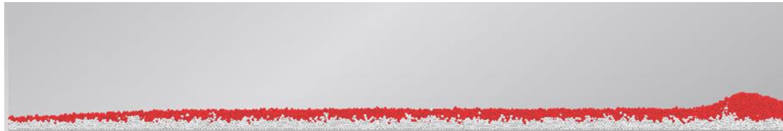
a) Final state, fill-level 30 mm (32490 particles) after single blade pass.
