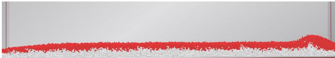
b) Final state, fill-level 42 mm (45480 particles) after single blade pass.
