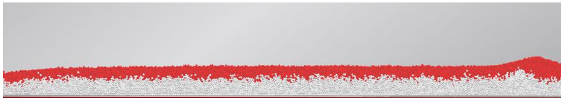
c) Final state, fill-level 59 mm (63890 particles) after single blade pass.
