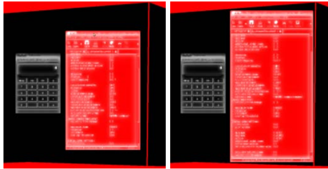
Figure 8.15: Screenshots of the resulting desktop importance map when maximizing a low-priority window in an irregularly shaped display region (display importance map of Figure 7.4): (a) the window layout before the maximize process, (b) and the resulting window layout, where the window to be maximized is squeezed between the calculator and the physical room corner.
