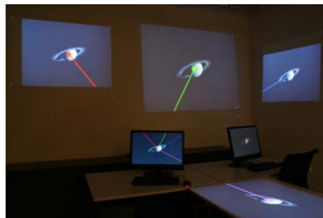
Figure 4.18: Visualization of the shortest paths from a start display (left monitor) to all possible target displays using a perspective mapping. Mind that the perspective plane corresponds to the camera position.
