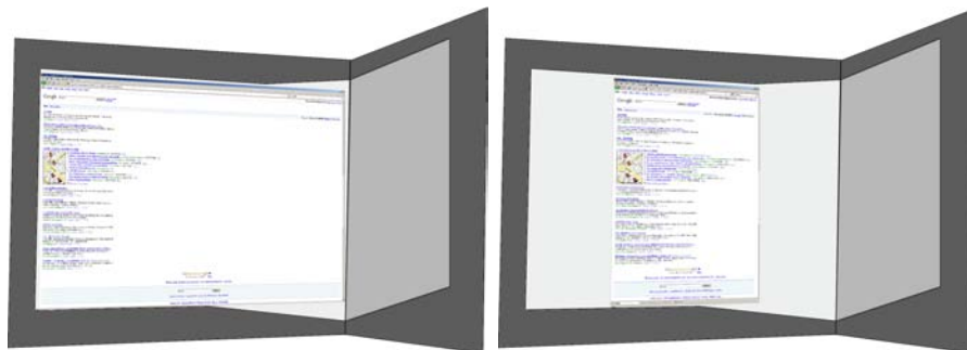
Figure 8.16: Conceptual sketch of content-adaptive maximize: (a) display-adaptive maximize finds the maximum window size with respect to the display outline; (b) adding content-adaptivity would furthermore restrict the window size if no more important information can be revealed when the window is enlarged.
