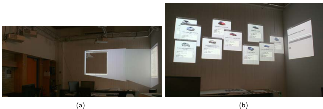
Figure 9.8: Irregular display setup for evaluation of display-adaptive window management: (a) the two projectors (on the left) driving the irregularly shaped display and (b) the resulting display with invisible outlines during the study.
