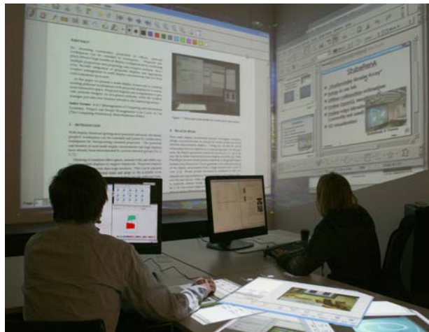
Figure 1.1: Multi-display environments combine projected displays and monitors of different size, resolution, and orientation into a common interaction space.
