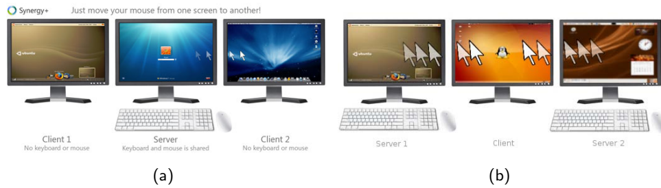
Figure 2.3: (a) A configuration of the original Synergy implementation: sharing a single mouse and keyboard pair across multiple machines and platforms ( http://code.google.com/p/synergy-plus/ ). (b) A possible configuration of Synergy+MPX with multiple mouse and keyboard pairs shared across multiple Linux machines.
