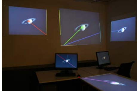
Figure 4.16: Visualization of the shortest paths from a start display (left monitor) to all possible target displays using pair-wise planar mappings and the A* search algorithm.
