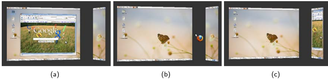
Figure 5.10: Window migration using the WIM control [24]: (a) the user can pick up a window at any location, (b) drag it to a remote display within the miniature view, and (c) drop it on a remote display. The window is resized to fit the display size. The window migration operation will be reflected in the “real” environment.
