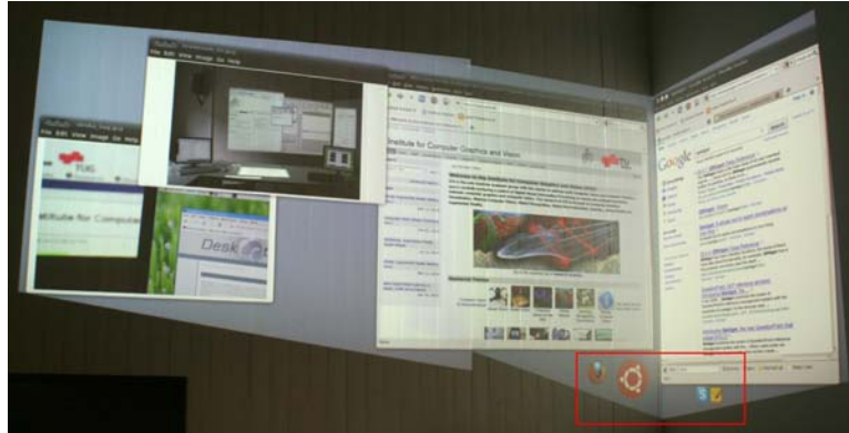
Figure 8.18: Desktop widgets on an irregular display are subject to semi-automatic window coordination and will therefore be moved to peripheral areas where no larger items can be reasonably placed.
