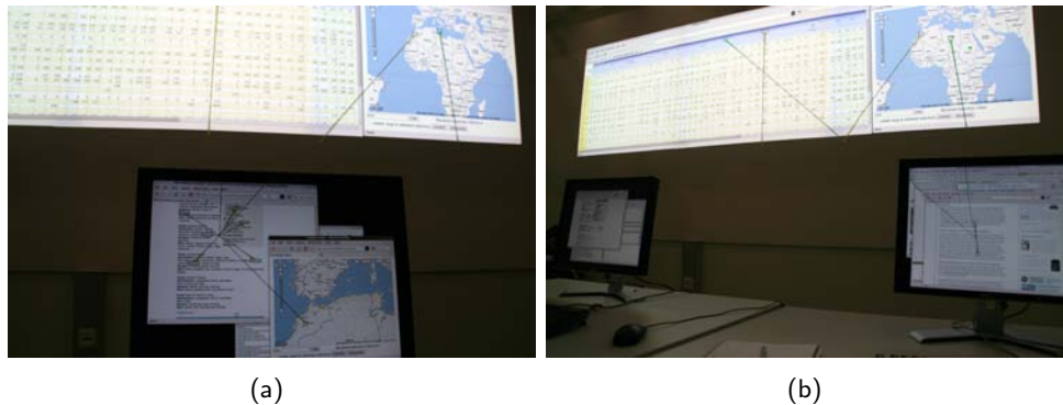
Figure 8.8: Cross-display links using a perspective mapping, as seen from the left (a) and right (b) user’s perspective. Even though the link colors are similar (yellow and green), the links can be discriminated based on their origin direction on the respective home display.
