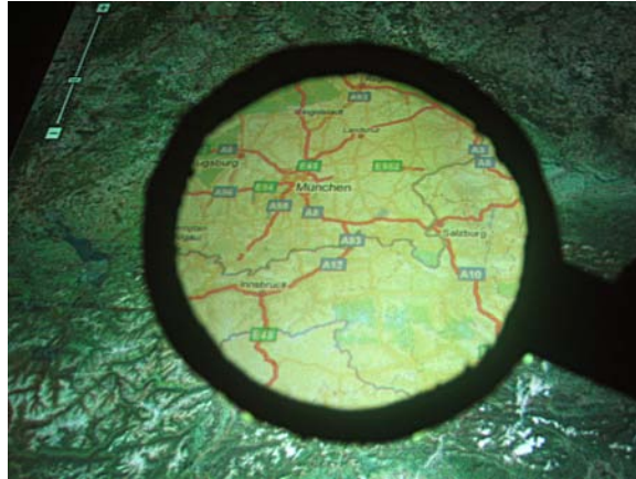
Figure 8.20: A satellite map view is locally filtered for a street map view.
