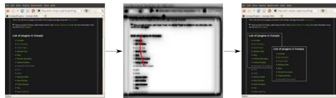
Figure 7.10: Conceptual sketch of semi-automatic region segmentation: on an application window, the user paints a rough stroke to indicate the region of interest. The segmentation is conducted on the window importance map. The duplicated window region can be treated as individual application window, as proposed by Tan et al. [238].
