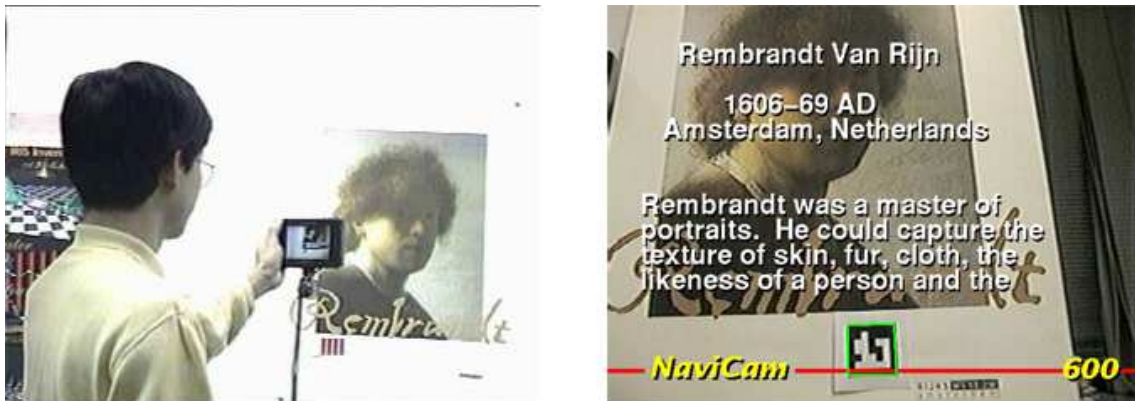
Figure 2.3: Rekimoto's Navicam (Left) used fiducial markers to register augmentations in the surroundings of the user (Right). [Rekimoto and Nagao, 1995]
