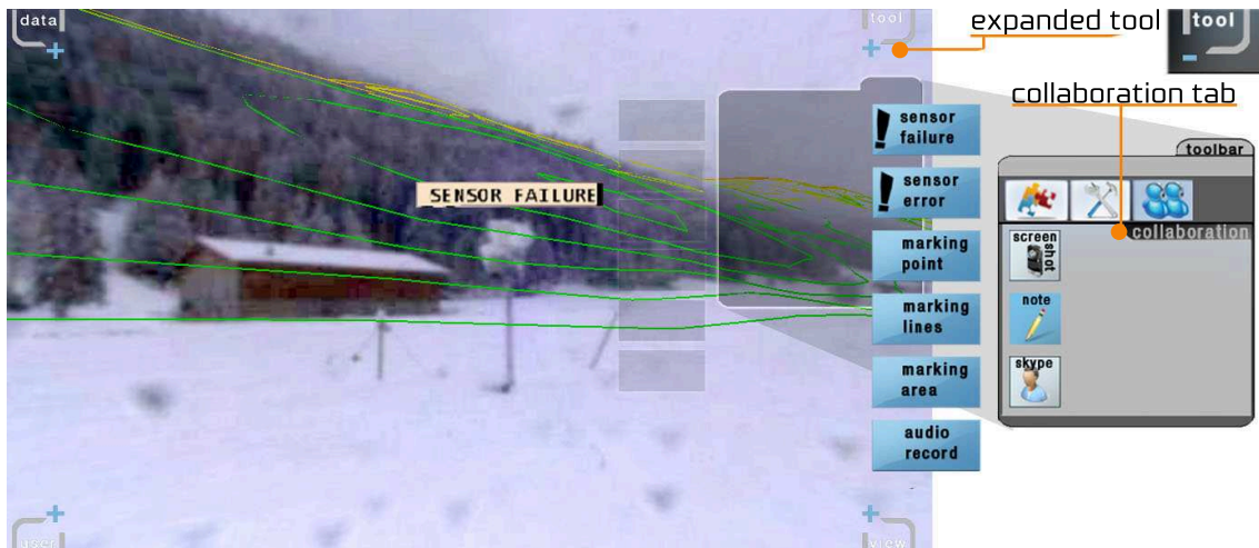
Figure 8.2: Collaboration Interface. The collaboration tab activates mechanisms to convey observations to peers, leaving annotations, or initiating real-time communication.
