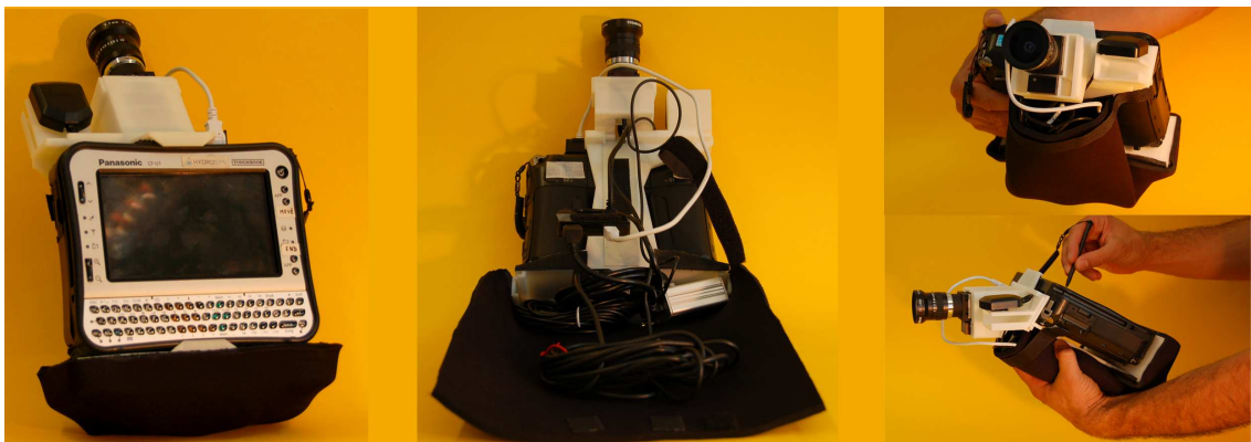
Figure 4.4: Cool'R: device with connected sensors, device taken apart showing different modular boxes, lens protection and open neoprene hull, and the single-handed pose with pen operation.
