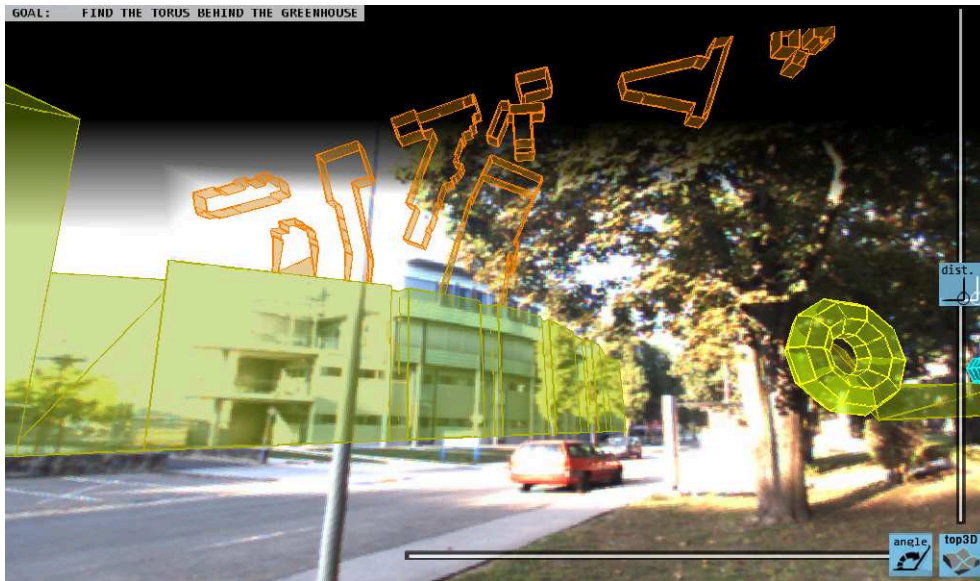
Figure 7.9: Variable perspective view. The video background is registered with its 3D representation from two perspectives.
