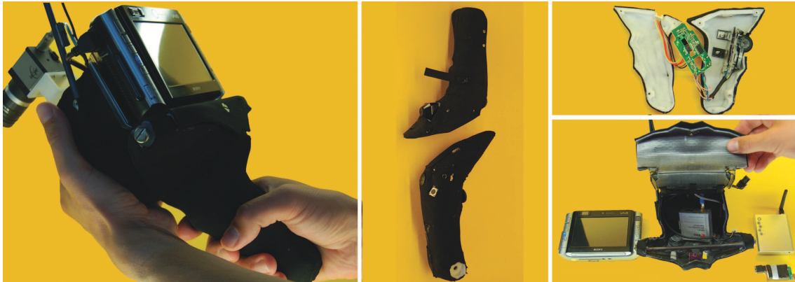
Figure 4.1: Vesp'R: the single-handed grip, the handles with different controllers, the inside of the new single-handed grip/handle and the backpack.
