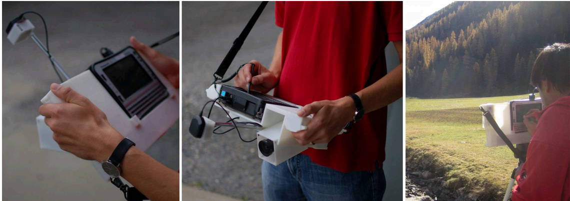
Figure 4.3: Ice'R: the different poses afforded by Ice'R, being two-handed at eye-height, single or two-handed with belt, and mounted on a tripod.
