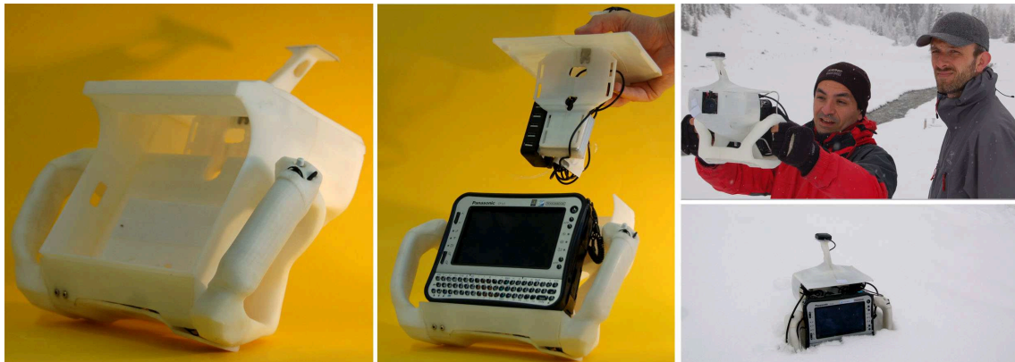
Figure 4.2: Bulk'R: the grip with the backpack, the fin construction for attaching devices and cables, and outdoor usage in harsh conditions.
