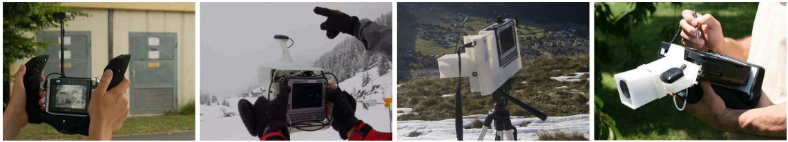
Figure 1.4: Four generations of handheld AR platform. (Left) Vesp'r design to explore spatial interaction and usage patterns. (Middle-Left) Bulk'r focused on robustness and weather-resistant construction. (Middle-Right) Ice'r aimed at compactness. (Right) Cool'r improved modularity and extreme weather resistance.
