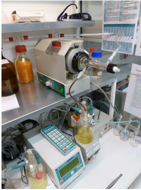
Figure D.2: Moisture determination of pressboard: a) Measurement set-up with KF Coulometer b) Weighing boat with sample in detail
