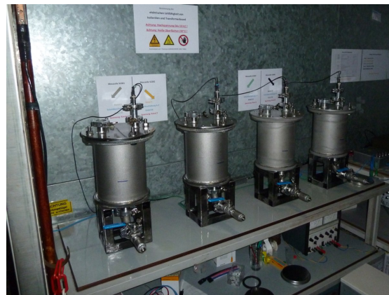
Figure 5.8: a) Schematic of conductivity measurement cell; b) Practical set-up
