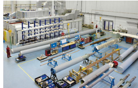
Figure 1.8: Schematic view of a HV condenser bushing core [58] Figure 1.9: Modern RIP HV bushing manufacturing [129]
