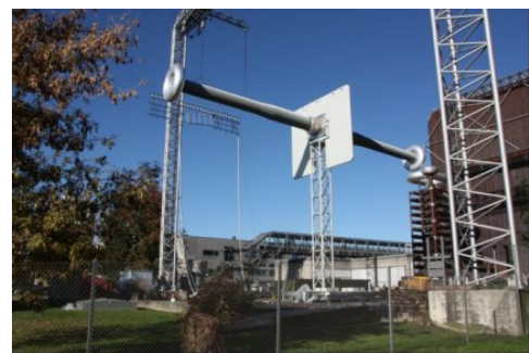
a) Figure 1.10: HVDC bushings for 800 kV systems during testing at Graz University of Technology: a) Transformer bushing 16 b) Wall bushing 16
