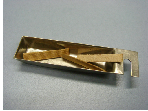
Figure D.2: Moisture determination of pressboard: a) Measurement set-up with KF Coulometer b) Weighing boat with sample in detail
