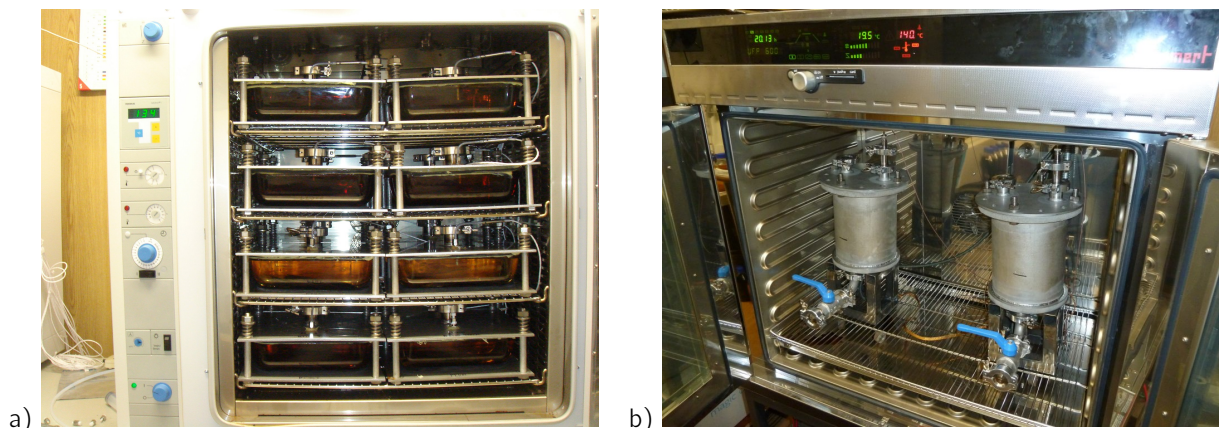
Figure 5.11: Thermal ovens with ageing vessels: a) Heraeus UT6200 with thermal ageing vessels; b) Mettmert UFP600 with combined ageing vessels
