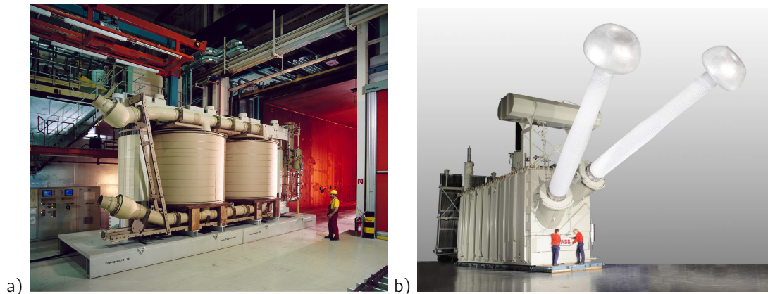
Figure 1.7: a) Active part of an HVDC converter transformer during manufacturing 14 b) Assembled HVDC converter transformer 15
