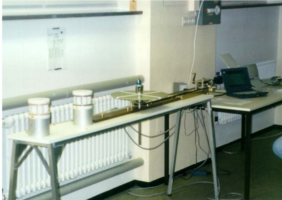
Figure 1.22. Gradiometer setup for magnetic measurements on spacecraft sub-systems (as used for the Rosetta Lander magnetic cleanliness program).
