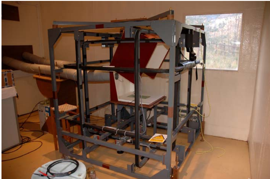
Figure 1.21. Helmholtz coil system for ground calibration (Photo: Imperial College, London).
