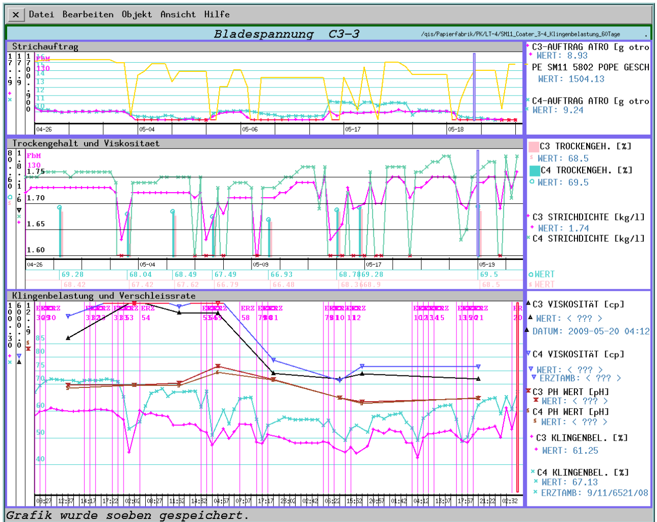
Pict. 10.7.3.9: Viscosity and blade load of middle coaters at OMC11 decreasing amount of caustic soda
