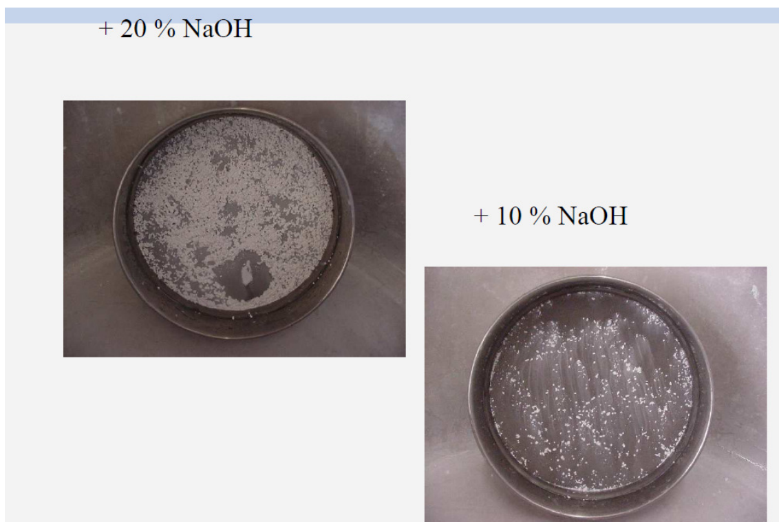
Pict. 10.7.3.7: Creation of pigment agglomerates by contact with too concentrated amount of caustic soda – residues on 45 µm screen (source: OMYA)
