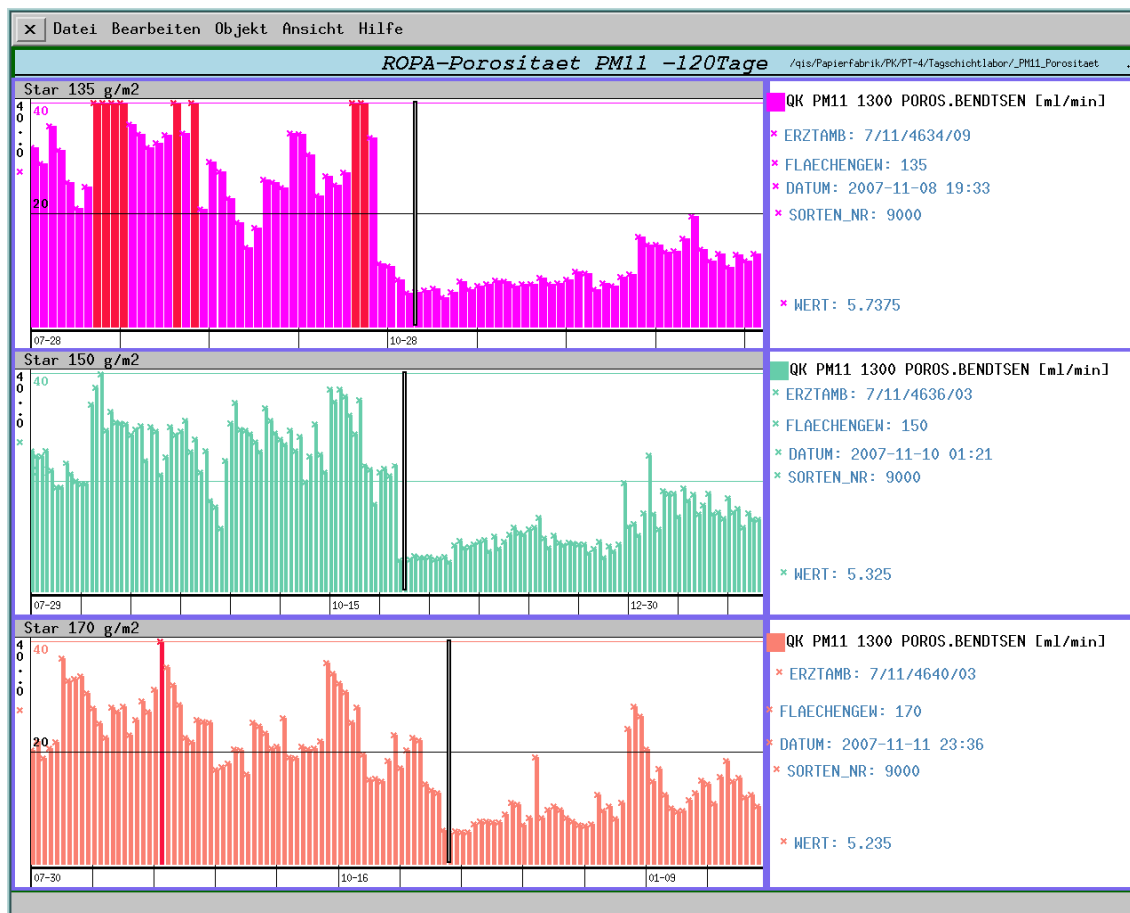
Pict. 9.5.11: Reduction of porosity of precoated paper by changing from 100% HC60 to 65% HC60 + 35% HC90
