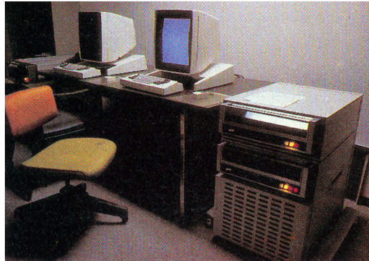
Figure 1.1: Xerox Alto. “Each Alto processor is made of medium- and small-scale TTL integrated circuits, and is mounted in a rack beneath two 3-megabyte hard-disk drives. Note that the video displays are taller than they are wide and are similar to a page of paper, rather than standard television screen.”
