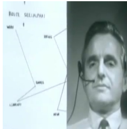
Figure 2.3: Douglas Engelbart during his demonstration of NLS. The variable split screen view allowed the audience to see the performer and the screen content. In this sequence, Douglas Engelbart showed a graphical representation of a travel plan which was enriched with hyperlinks on each node containing a hierarchical shopping list. [Video Screenshot]
