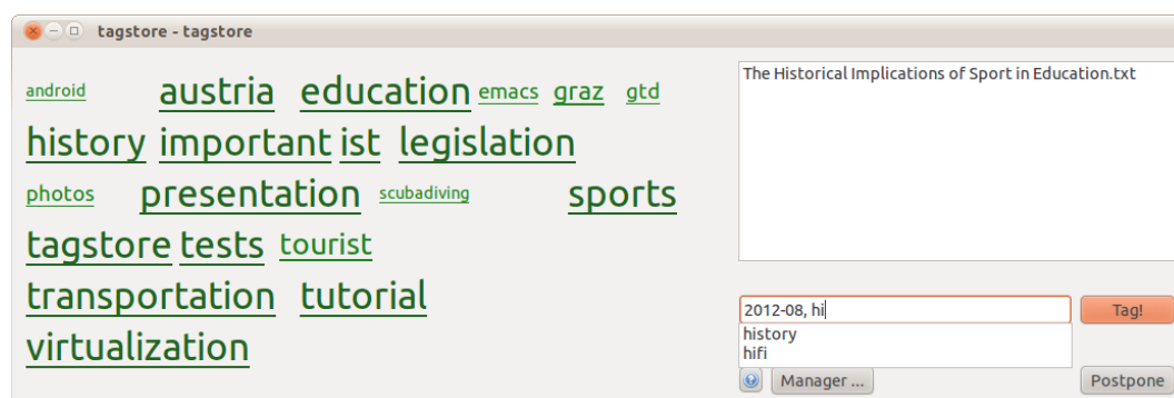
Figure 5.2: A screenshot of the tagstore tagging dialog from the 2012-08-16 version using GNU/Linux. On the right-hand side, the list shows all untagged items that are stored in the storage folder. On the bottom right side, the user can enter comma-separated tags into the tag line. The tag-recommending feature shows the two possible completions for partially typed-in string “hi”. The left side consists of tag recommendations from the recommender system.
