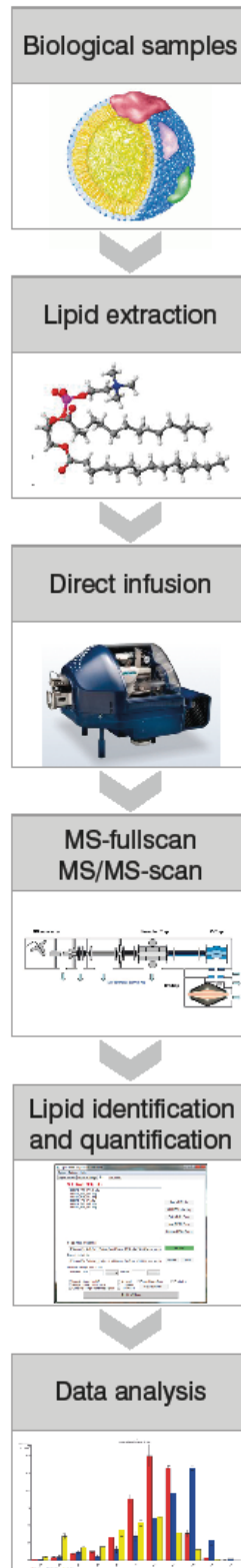
Figure 1. Schematic outline of a high throughput shotgun lipidomics platform consisting of an LTQ-Orbitrap mass spectrometer coupled to a NanoMate.
