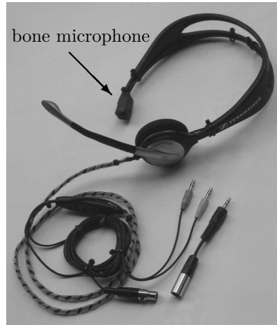
Figure 4.1: Headset with integrated bone conduction microphone [71].
