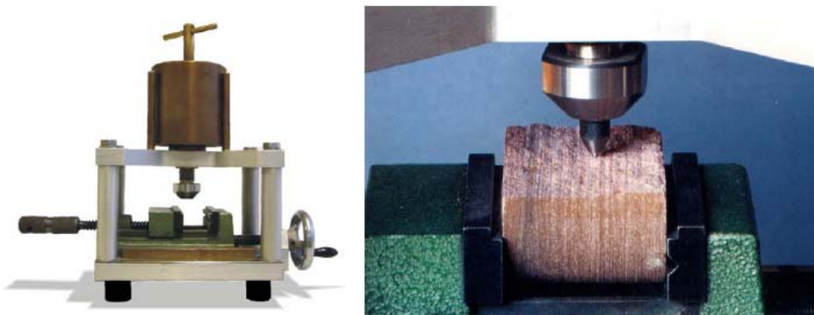
Fig. 30: Cerchar test – test device according to West (1989) (left) – rock sample with testing pin (from Plinninger (2007))
