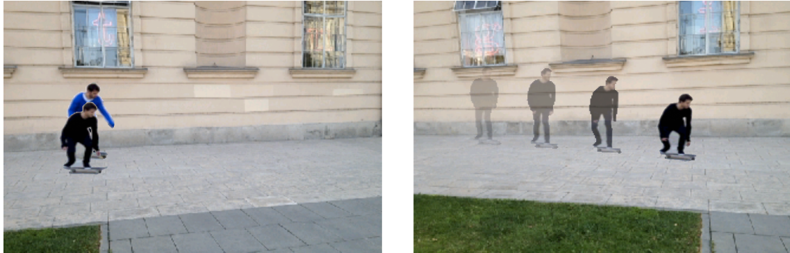
Figure 6.12: Examples of layers and an example of realized post effects as used in our skateboard tutor application as captured from an iPhone 4. (Left) Playing back two video augmentations layers allows the comparison of the riders' performance. (Right) Flash-trail effects visualize the path and the motion within the video.
