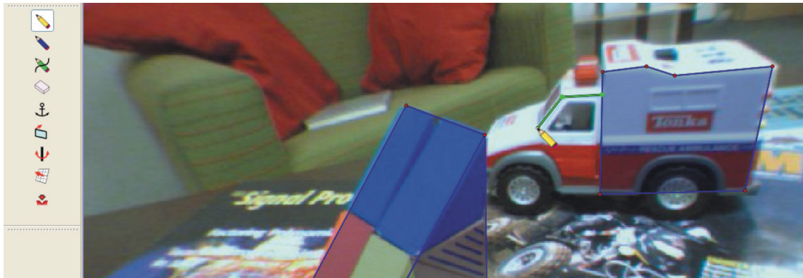
Figure 2.11: In-situ image-based modeling. The system allows automatic extrusion of selected image areas for creating 3D models of existing objects [143].
