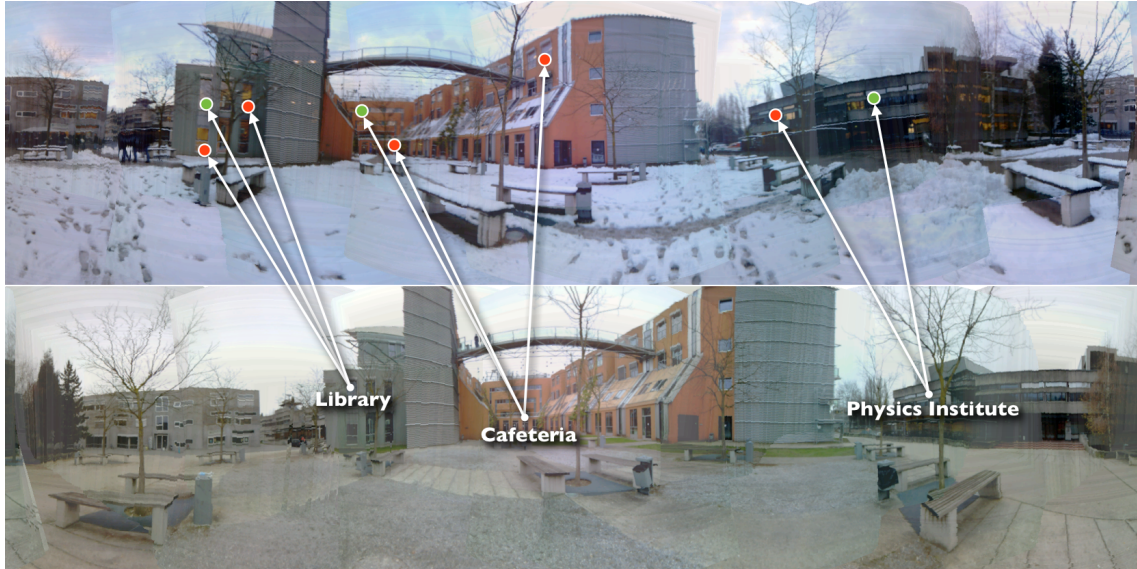
Figure 5.10: A source panorama that was used to create the annotations. (Top) A newly created panorama with the best candidates for placing the annotation resulting from the template-based matching. For every annotation anchor point, we store a maximum of three best matches. The green dots in the upper image have the best matching scores and are therefore used for label placement. The red ones are the second and third best matches of an annotation, which makes them a candidate for a possible correct match.
