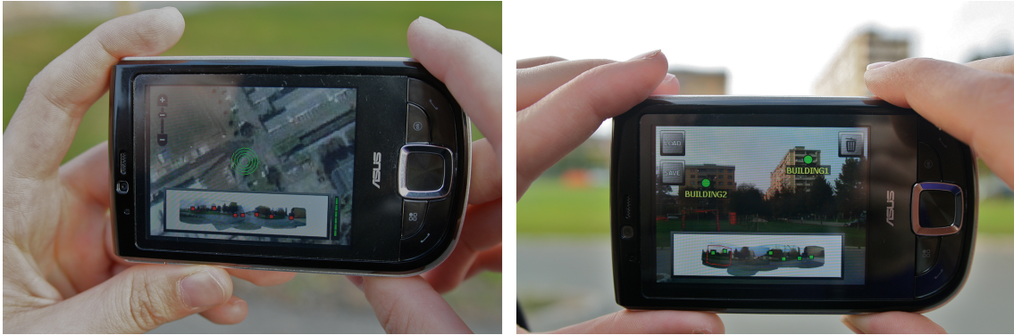
Figure 5.5: (Left) 2D map overview showing nearby annotations. (Right) First-person view of the annotated panorama.
