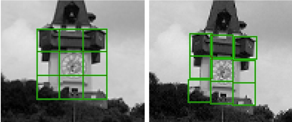
Figure 5.4: The support area of an annotation is described using a 3x3 grid of templates encoded using a Walsh transform. (Right) Matching the templates from a slightly different camera perspective.
