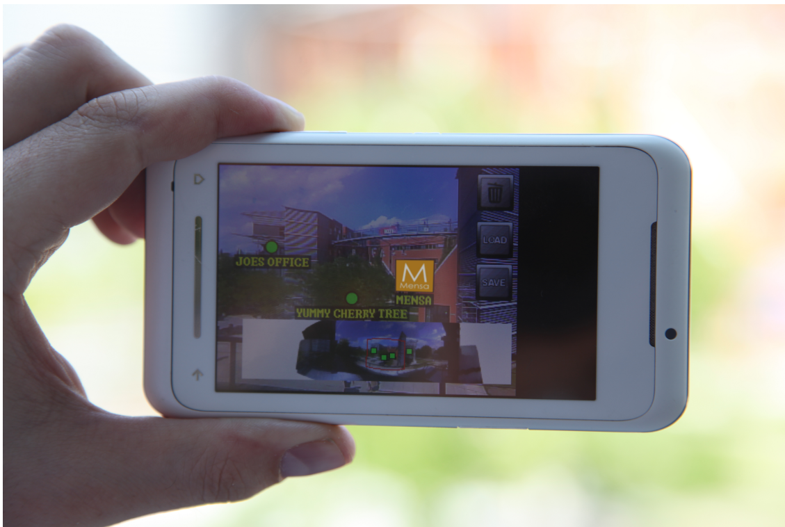
Figure 5.2: Implemented prototype showing panorama-referenced 2D annotations and a partially recorded panorama that is used for tracking and matching the annotations.
