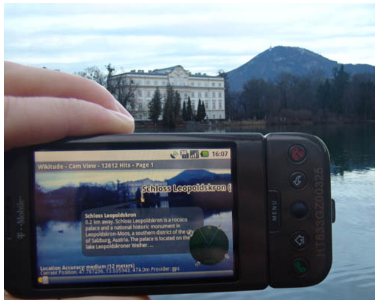
Figure 2.4: Wikitude, the first commercial AR browser running on the T-Mobile G1
