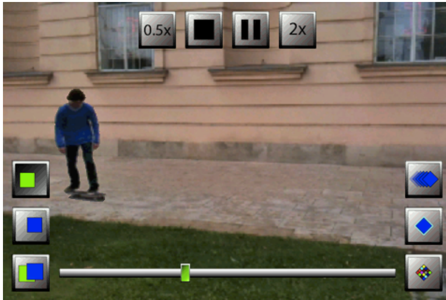
Figure 6.11: Screenshot of our prototype showing a video augmentation together with the control groups for video control (top and bottom), video layers (left side) and video effects (right side).
