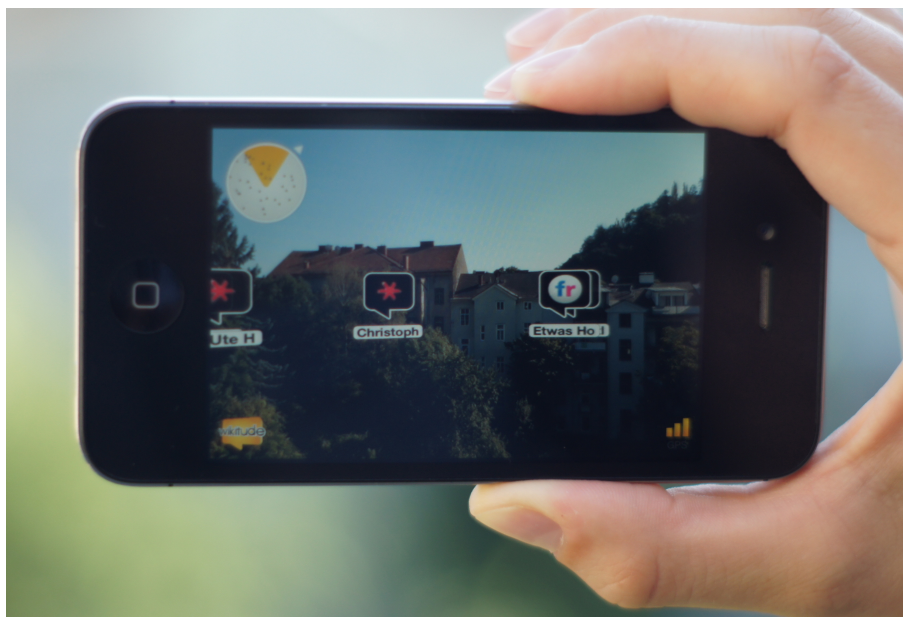
Figure 1.1: Wikitude, the first commercial AR browser application as an example of an AR-based personal information system running on a smartphone.
