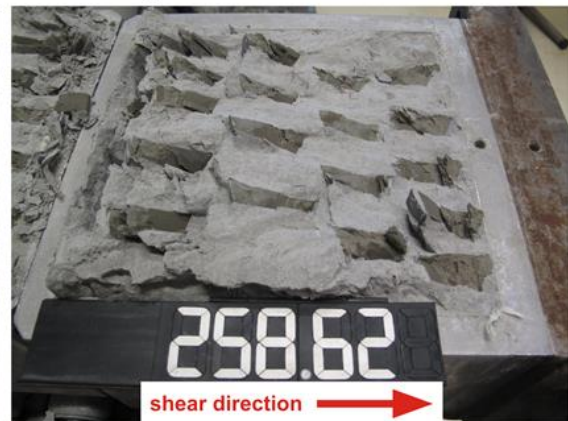
upper shear surface after the test
