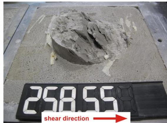
upper shear surface after the test
