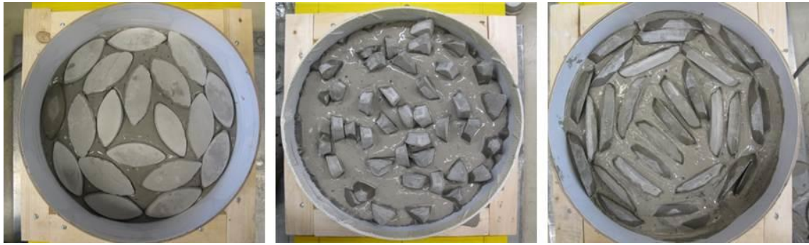
Figure 59: Sample preparation for large oedometer tests; blocks horizontally aligned (left), blocks vertically aligned (middle), blocks twisted (right).
