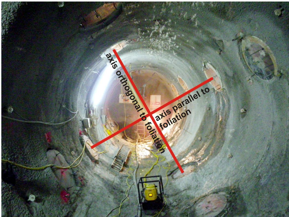
Figure 22: Positioning of the measurement axis, adjusted to the foliation.
