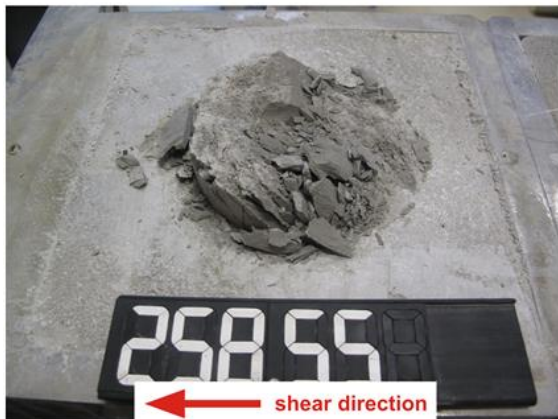
lower shear surface after the test
