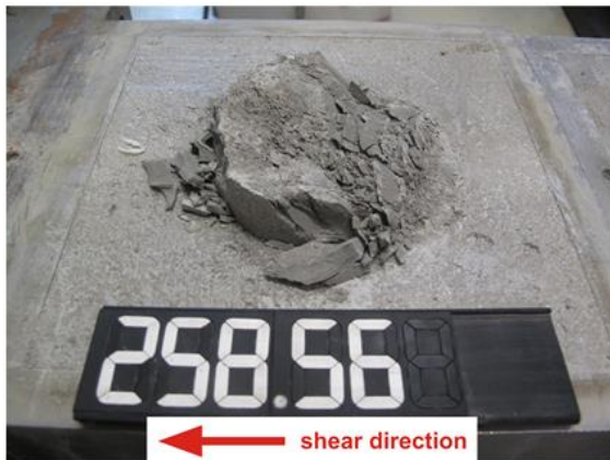
lower shear surface after the test
