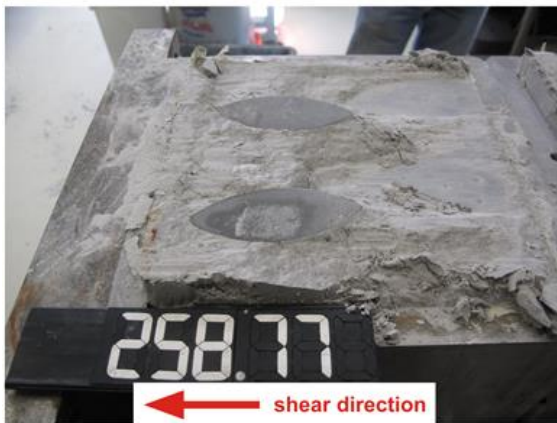
lower shear surface after the test
