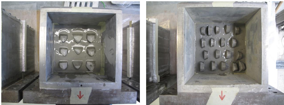
Figure 83: Assembly of the shear boxes, lower box filled with matrix material and blocks attached; exemplarily shown for 25% block proportion/30° block orientation (left) and 50% block proportion/90° block orientation (right).
