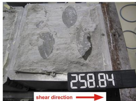
upper shear surface after the test
