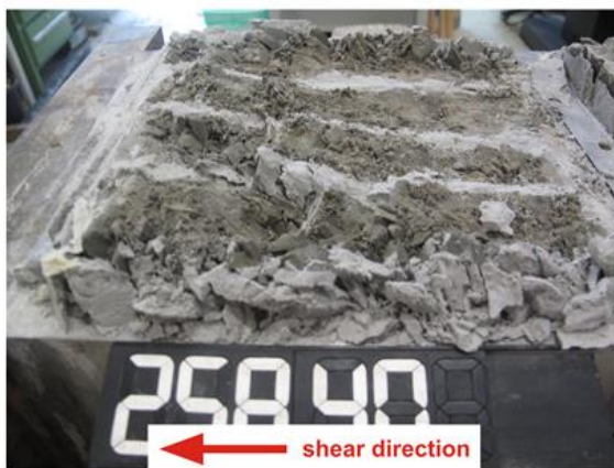
lower shear surface after the test
