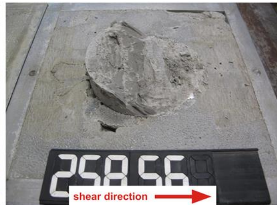
upper shear surface after the test
