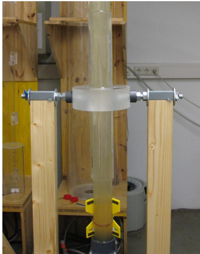
Figure 4.17: Assembly for holding the settling column
