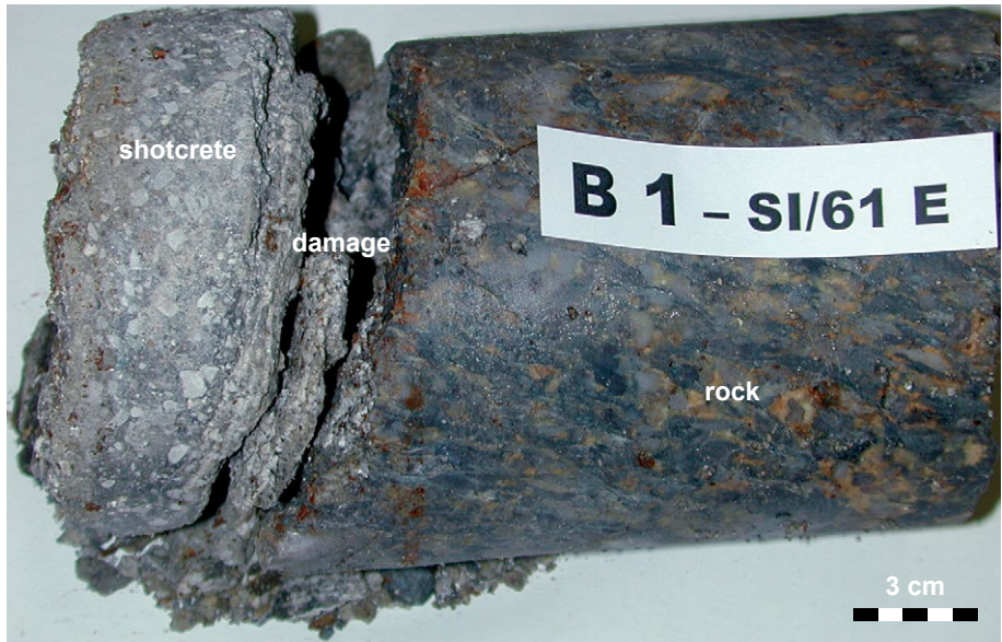
Figure 1: 100 mm \varnothing drill core from a shotcrete with damage due to sulfate attack.
