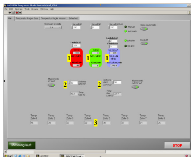
Figure 3.14 Graphic surface with (1) Massflow controller that changes the flow for H 2 / air (O 2 ) / N 2 , (2) Display of the temperature for the inlet gases and (3) Display for the cell temperatures
