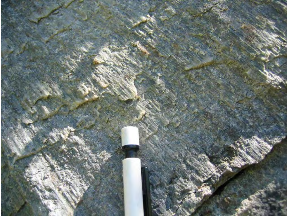
Figure 3-9: Calcite fibres on fault plane in a marble quarry near Twimberg (Carinthia) with a sinistral sense of shear (missing block downwards to the right), orientation of plane is 278/84 with striation 194/45. For location refer to Figure 3-17 a, outcrop ID is 175.
