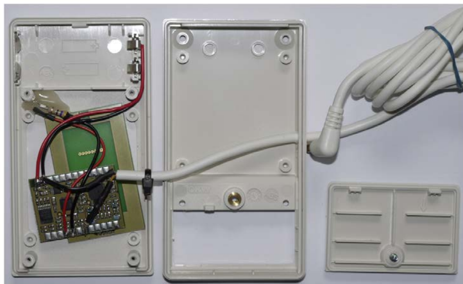
Figure 4: An opened KIT box with an integrated NFC module and RFID tag.
