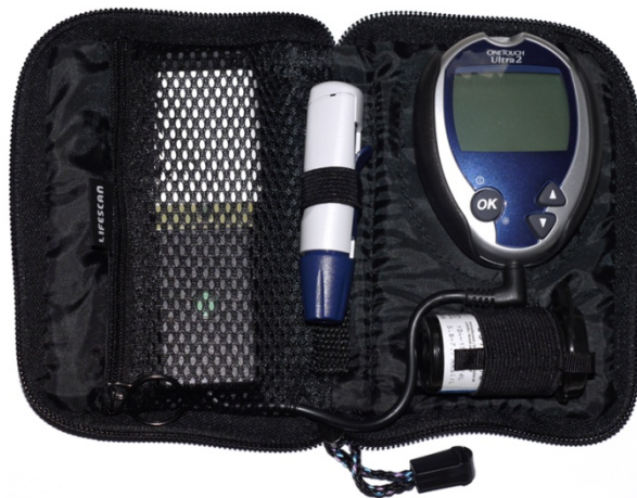
Figure 6: Bag with inserted blood glucose meter OneTouch Ultra II and connected KIT box.
