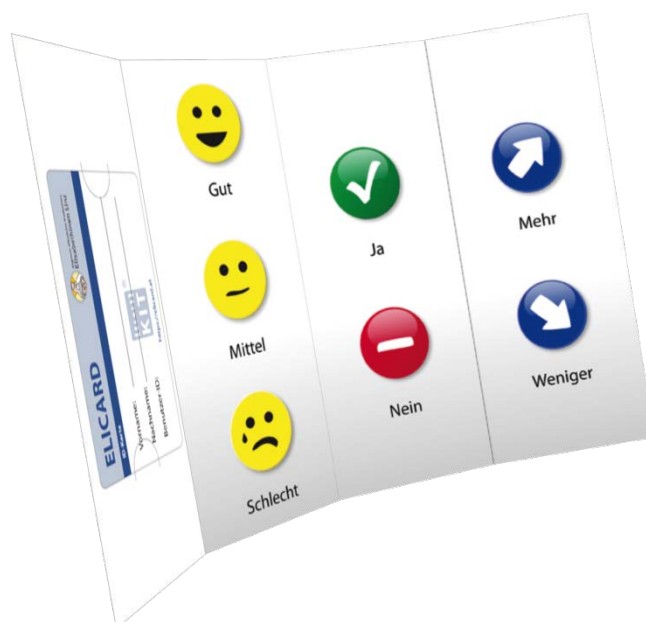
Figure 9: A dialogue book with icons and RFID tags to be touched for answering questions displayed on the mobile phone. The yellow icons were used to indicate the well-being state or subjective pulmonary functions (good, medium, and bad), the meaning of the green, red, and two blue icons was yes, no, more, and less, respectively;
