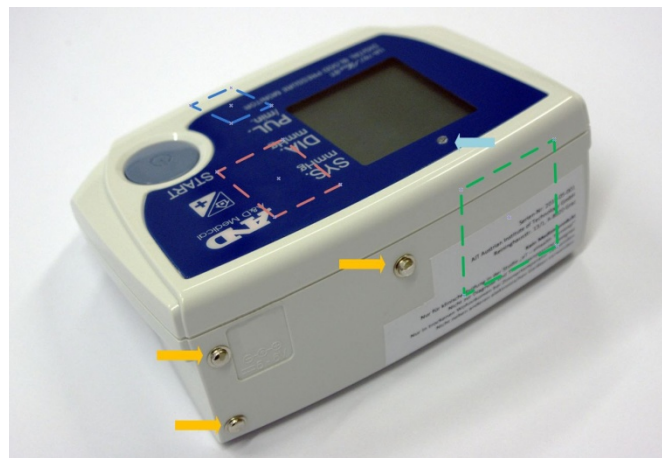
Figure 8: Modified blood pressure meter with three electrodes (orange arrows), integrated microcontroller with ECG amplifier (green square), Bluetooth module (blue square), RFID tag with field detector (red square), and light emitting diode (light blue arrow).
