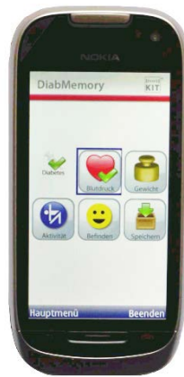
Figure 7: Nokia 701 with running MobileMonitor: green checkmarks indicate that data have been acquired and are ready for synchronization.
