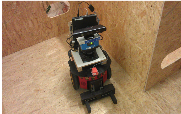
Figure 10.5: Pioneer 3DX robot equipped with Laser and IMU sensors.
