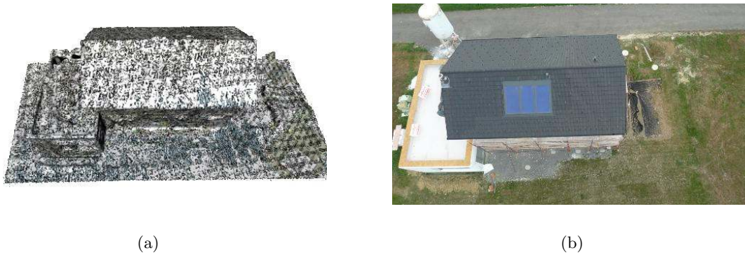
Figure 6.31: Comparison of planned view and approached position. View (a) is rendered from the desired viewpoint, but the image taken by the MAV in (b) shows a slightly different part of the scene. The two poses mainly differ by a translation along the building caused by noisy GPS positions.
