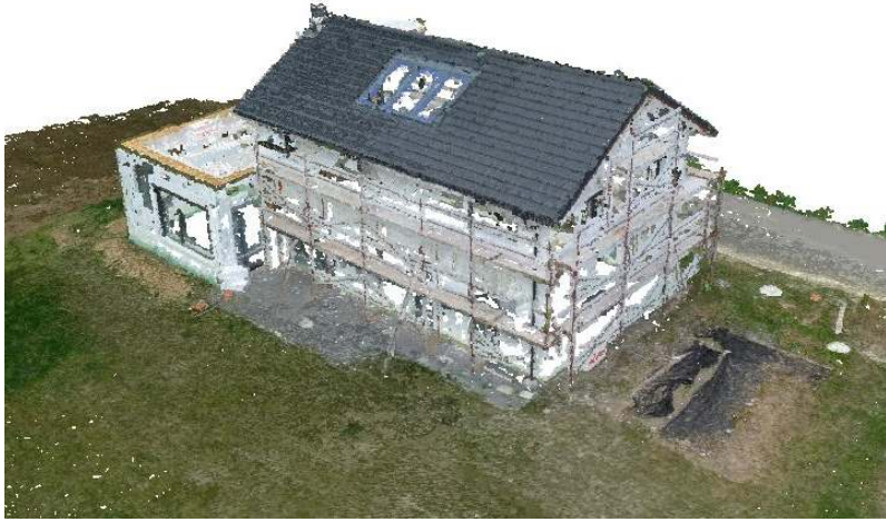
Figure 6.32: Densified reconstruction after executing an autonomous flight plan. This result is achieved by using patch-based densification [65]. The missing parts of the facade are caused by weak texturing.
