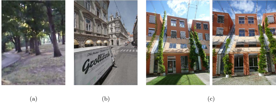
Figure 2.2: Degenerate structures in visual SLAM. (a) Indiscriminative features, (b) loss of tracking due to sudden occluders, (c) and repetitive scenes are just some examples for situations which cause problems when creating visual maps online.
