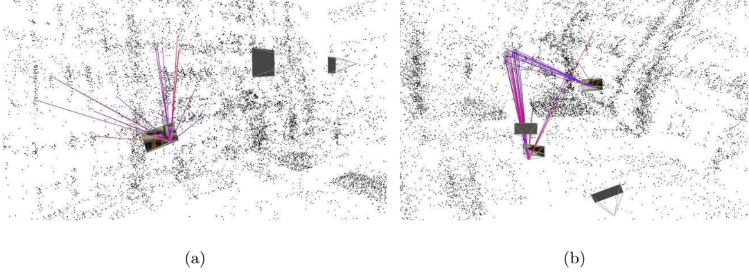
Figure 4.12: Localization initiated by virtual cameras. (a) In most cases, pose estimation based on the virtual cameras V_t^{1:3} (visualized without texture) results in the same final absolute pose P_t (textured with the query image). (b) If the results do not coincide, the pose P_t with most effective inliers I_{eff} (red matches) is preferred to other poses (blue matches).
