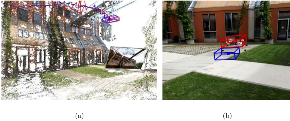
Figure 6.19: Visual comparison of the localization results based on a registered groundtruth video. (a) Oblique view of registered groundtruth showing the current camera frame and MAV positions (path and bounding box) estimated by our localization approach (red) and the aligned PTAM result (blue). (b) Back-projected bounding box from the observer’s point of view.
