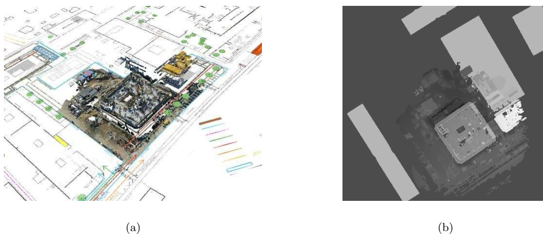
Figure 4.9: Providing context in visualization. (a) A construction site aligned to a construction plan using an estimated DSM. (b) The estimated DSM can be enhanced by fusing the aligned model into it.
