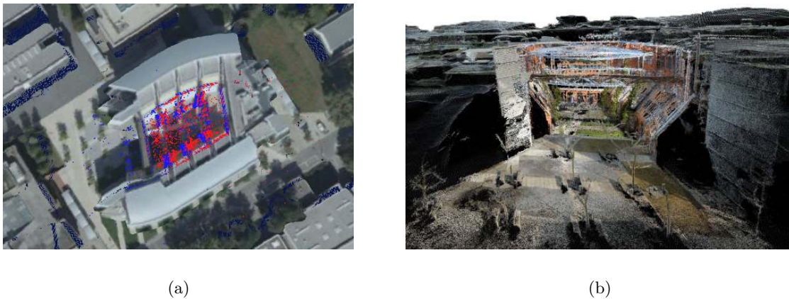
Figure 4.8: Season-invariant matching. (a) Accurate alignment allows to collect local features in different seasons (blue, red) and fuse the overlapping point clouds. (b) The aligned models have been acquired in different seasons (summer and winter), as can be seen when looking at the vegetation. While the appearance differs, the alignment in a global coordinate system is successful.
