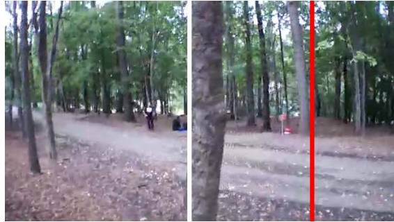
Figure 5.10: Usability challenges. In this exemplary frame from the MAV camera stream, the white line indicates the yaw commanded by the current DAgger policy \pi_{n-1} while the red line indicates the yaw commanded by the expert. In this frame DAgger is wrongly heading for the tree in the middle while the expert is providing the correct yaw command to go to the right instead. These expert controls are recorded for training later iterations but not executed in the current run.
