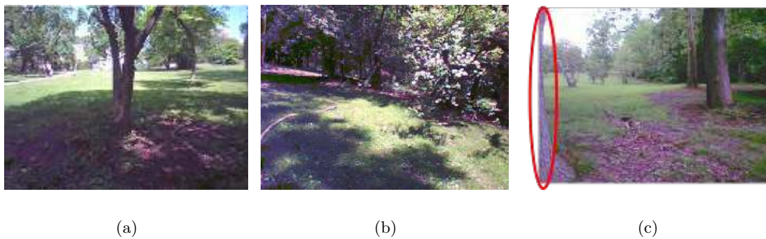
Figure 6.38: Typical failures during training iterations. While the controller has problems with tree trunks during the first iteration (a), this improves considerably towards the third iteration, where mainly foliage causes problems (b). Over all iterations, the most common failures are due to the narrow FOV of the camera where some trees barely appear to one side of the camera or are just hidden outside the view (c). When the UAV turns to avoid a visible tree a bit farther away it collides with the tree to the side.
