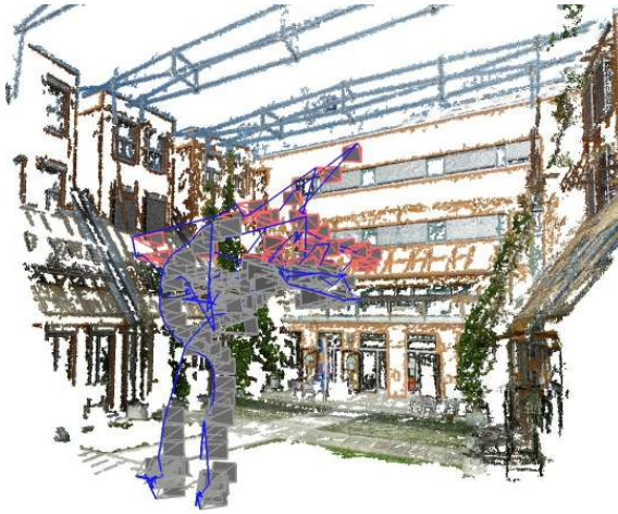
Figure 6.17: Visual localization result for an entire MAV flight. In a non-adaptive setting, we can localize 62.8% of all frames of this dataset (gray camera positions). By using our technique of incremental feature updates, we are able to boost the localization performance to 83.1%, especially for high-altitude views (red camera positions).
