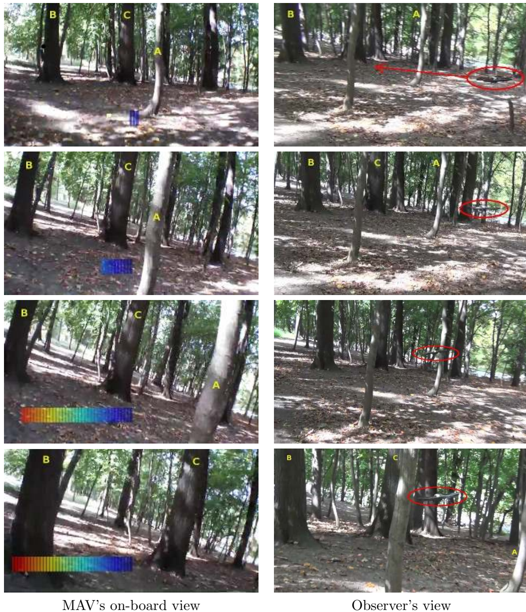
Figure 6.41: Example flight in a dense forest area. The image sequence is chronologically ordered from top ( t = 0s ) to bottom ( t = 2.9s ) and split into the MAV's on-board view on the left and an observer's view to the right. Note the direction label of the MAV in the first frame, and the color-coded commands issued by DAGGER. It can be observed that after avoiding tree A in frame 3 the vehicle still rolls strongly to the left in frame 4. This is due to the small but ubiquitous latency and should be addressed in future work to fly the MAV in even denser areas.
