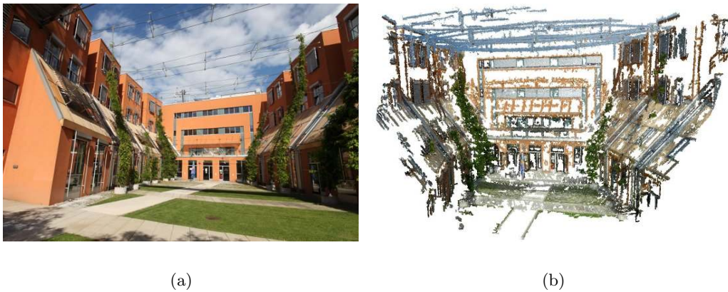
Figure 3.10: Densified atrium scene reconstruction. (a) Original view of the scene. (b) Semi-dense point model obtained by refining the sparse atrium model with PMVS [65].
