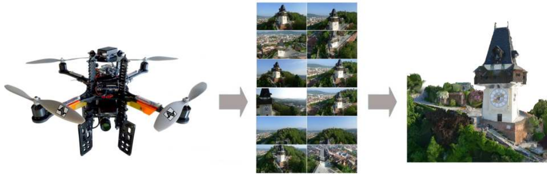
Figure 1.1: Reconstruction of the clocktower in Graz, Austria. An MAV allows to acquire imagery from new points of view which cannot be reached otherwise. The imagery can then be used for 3D reconstruction to visualize landmarks, for inspection of industrial structures, for photogrammetrical measurements, or as maps for autonomous navigation.
