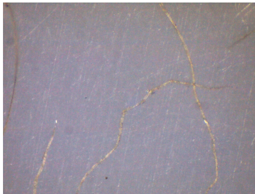
Figure 3.20 Fiber to fiber joint on teflon foil
