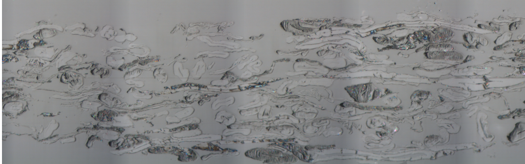
Figure 5.18 Paper cross section after microtome cutting (Lorbach, C., personal communication, January 23 th , 2013)
