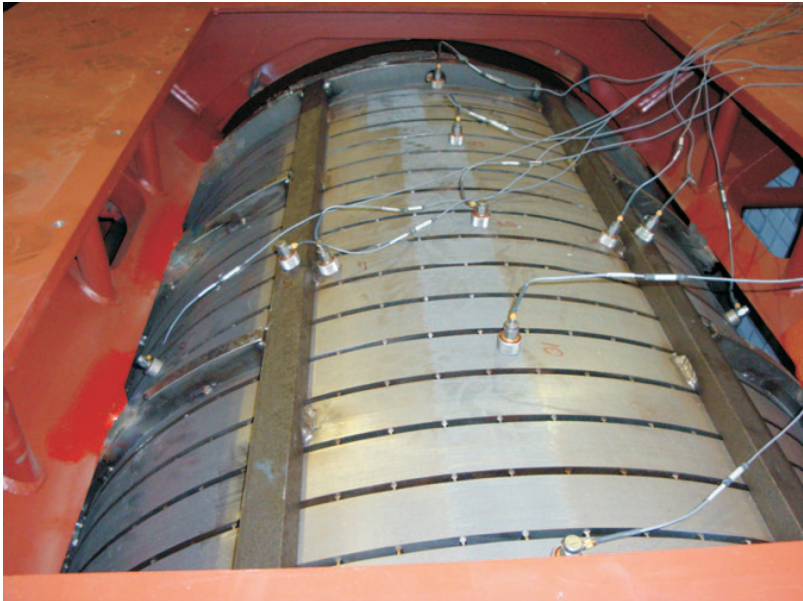
Figure 5.8: Measurement assembly - placement of the acceleration sensors on the surface of the investigated stator core stack
