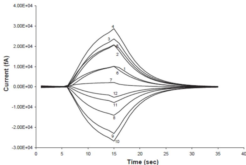
Figure 3.10: Charge profile of a typical actuation from a MDI [129]
