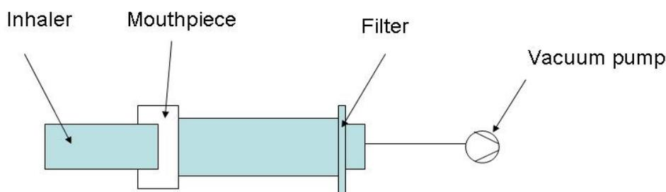
Figure 5.2: Experimental Set up, Flowability
