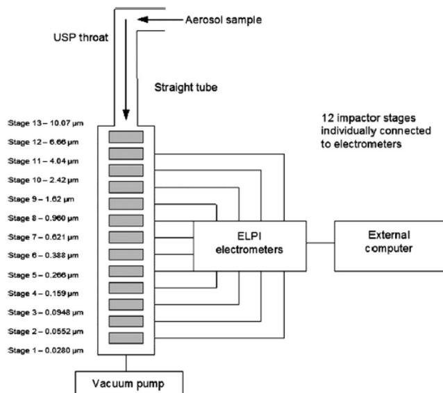
Figure 3.9: Schematic diagram of an ELPI [67]
