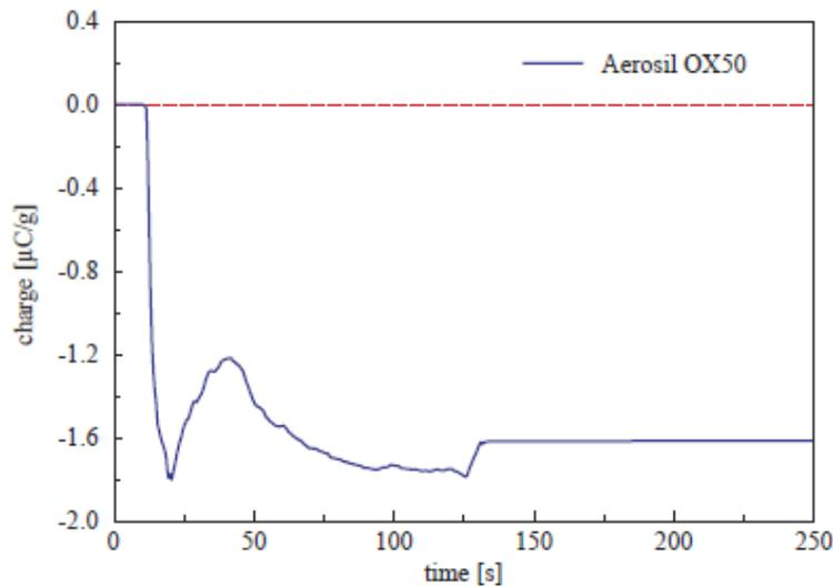
Figure 3.2: Electrostatic charge of Aerosil OX50® during dispersing [35]
