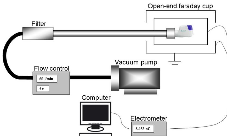
Figure 7.1: Schematic illustration of the experimental measurement setup
