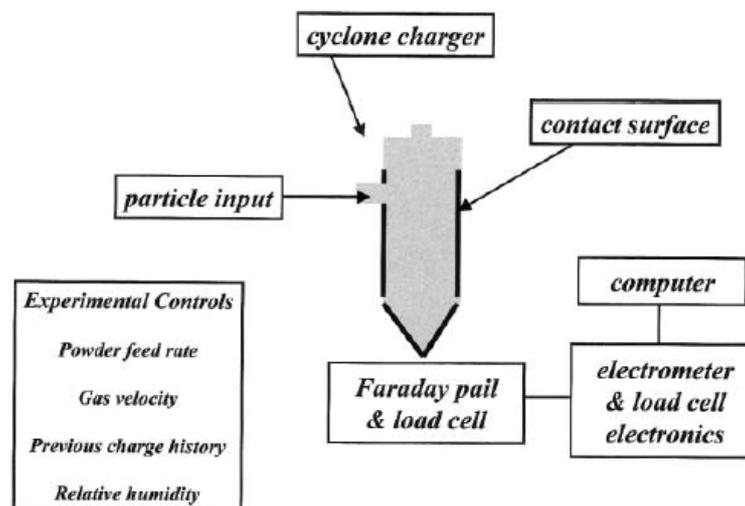
Figure 3.3: Sketch of a cyclone charger setup [38]
