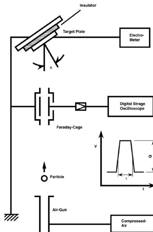
Figure 3.7: Schematic illustration of the single impact experimental set-up [26]
