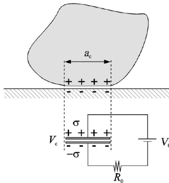
Figure 3.1: Capacitor model of contact charging [25]
