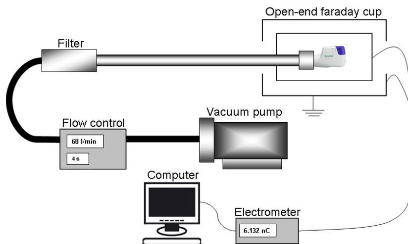
Figure 6.2: Schematic illustration of the experimental measurement setup
